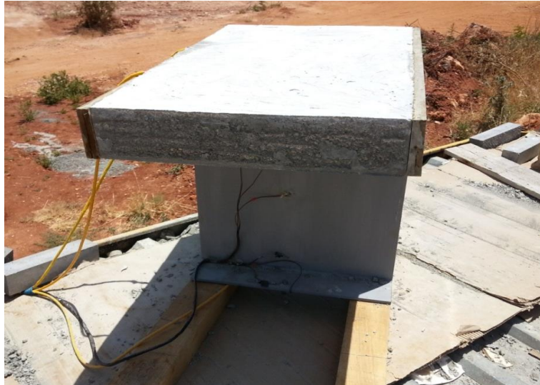
Figure 3.17 The T-Beam specimen after casting.
