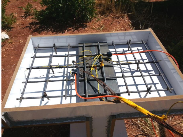
Figure 3.25 Sensor and measurement devices set up in I-Beam specimen.
