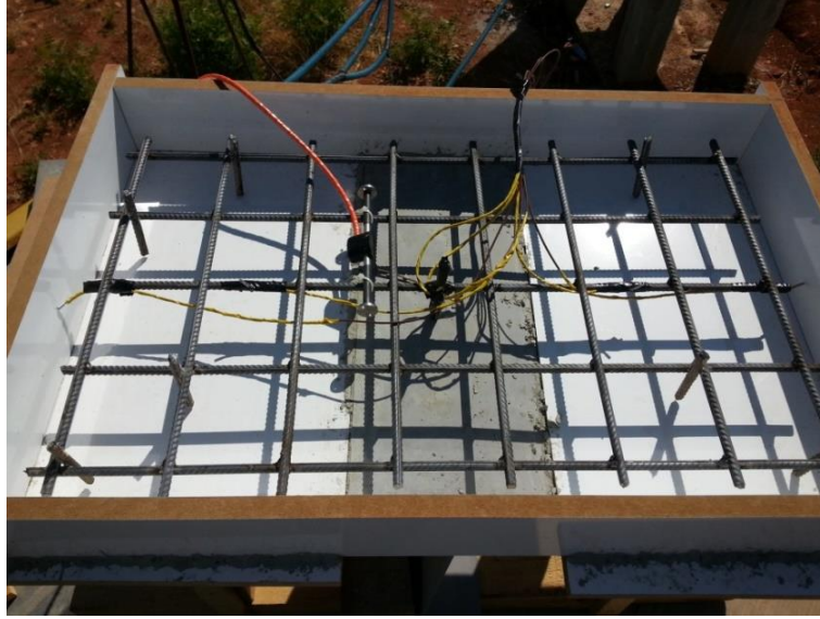
Figure 3.24 Sensor and measurement devices set up in the T-Beam specimen.
