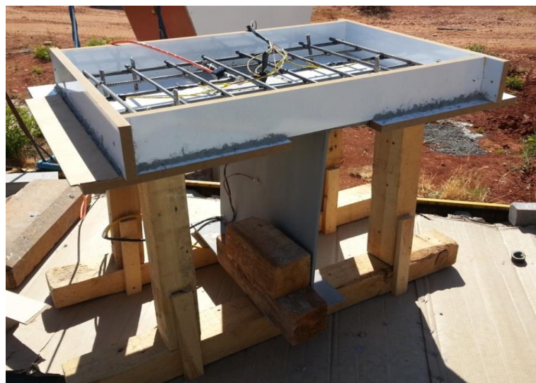
Figure 3.16 The T-Beam specimen before casting.
