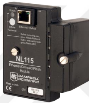
Figure 3.10 The L115 Ethernet/ compact flash module.
