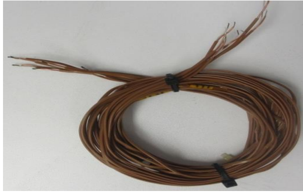
Figure 3.11 The thermocouple type T.
