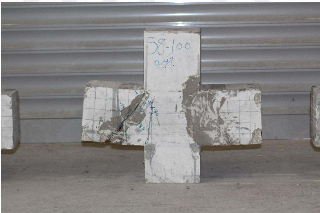
Figure 4.38 Unconfined (Specimen S8 - 100 - 0.4%) after testing
