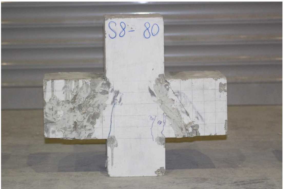
Figure 4.50 Unconfined (Specimen S8 - 80) after testing
