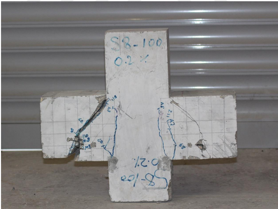
Figure 4.17 Unconfined (Specimen S8 - 100 - 0.2%) after testing
