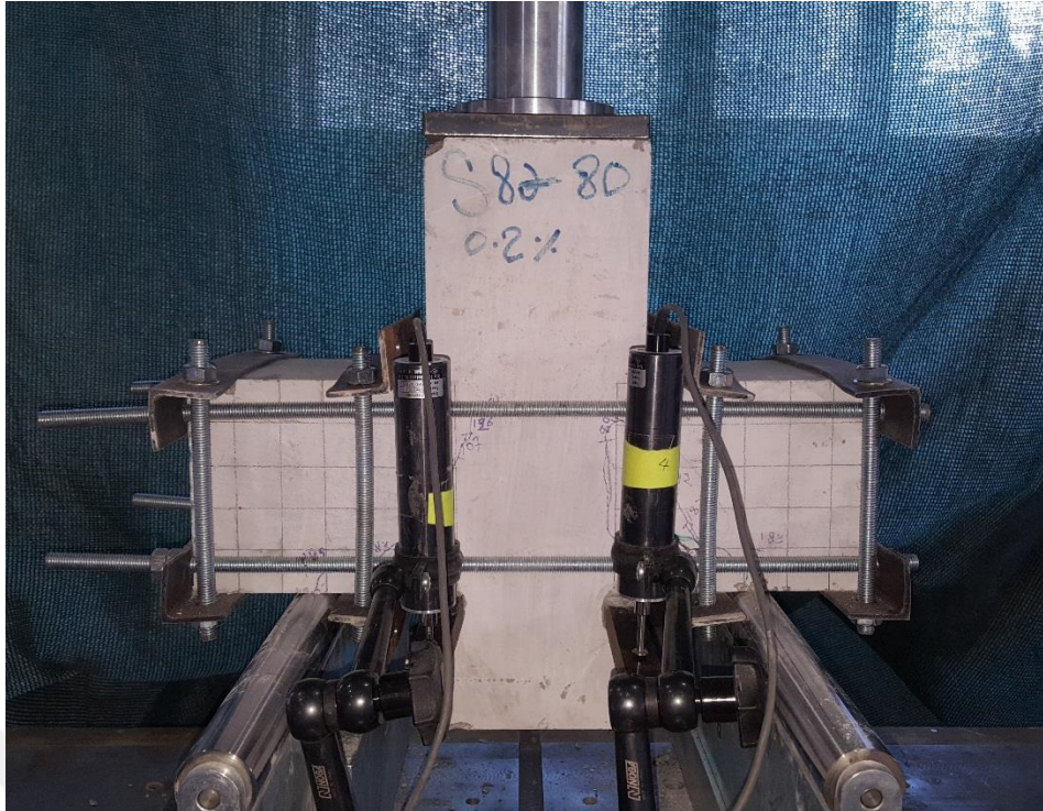
Figure 4.22 (Specimen S8 - 80 - 0.2%) in the test machine
