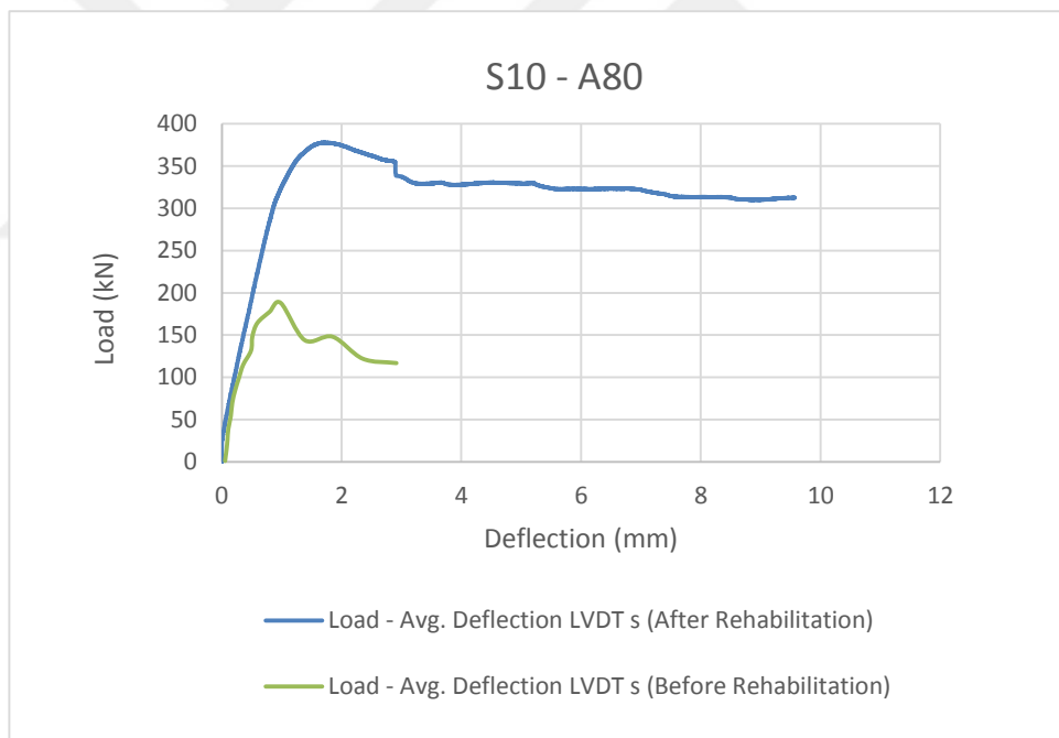
Figure 4.57 Effect of rehabilitation, style-4 (Specimen S10 – A80)
