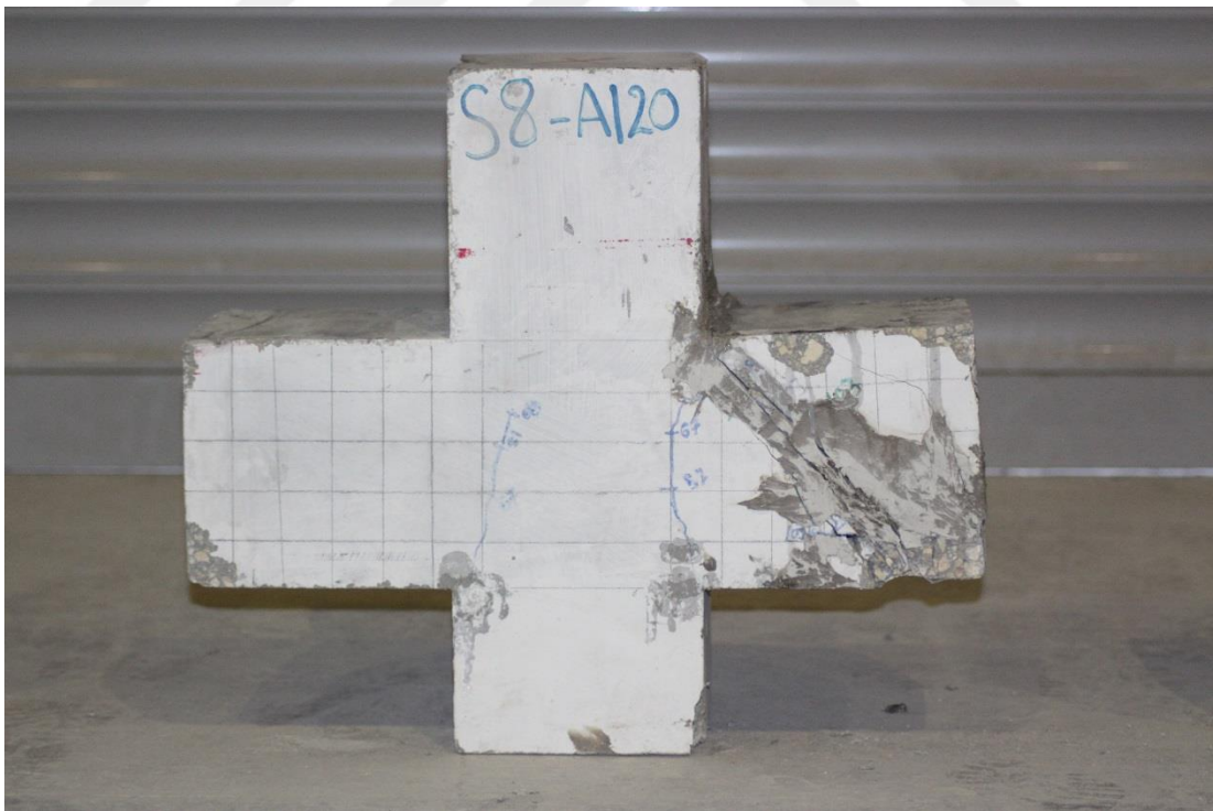
Figure 4.29 Unconfined (Specimen S8 - A120) after testing
