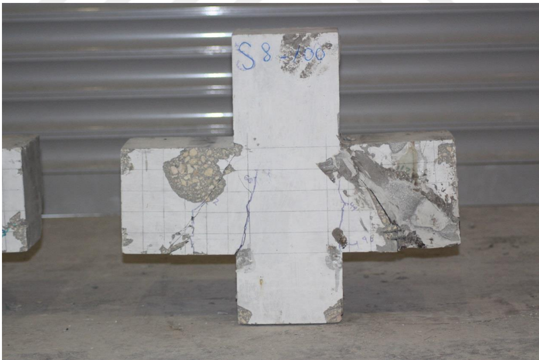
Figure 4.35 Unconfined (Specimen S8 - 100) after testing
