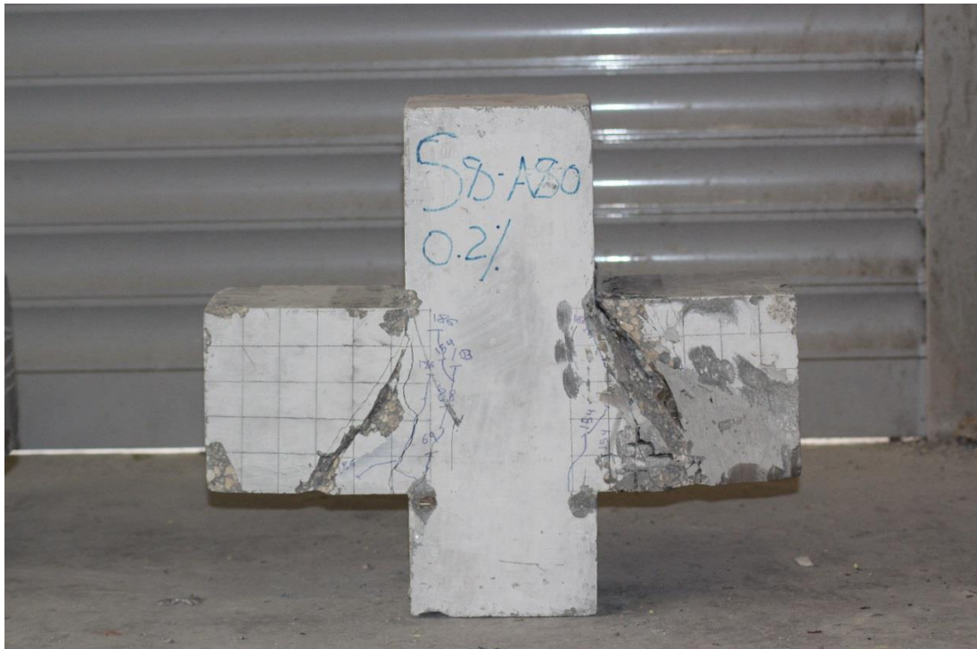
Figure 4.44 Unconfined (Specimen S8 – A80 – 0.2%) after testing
