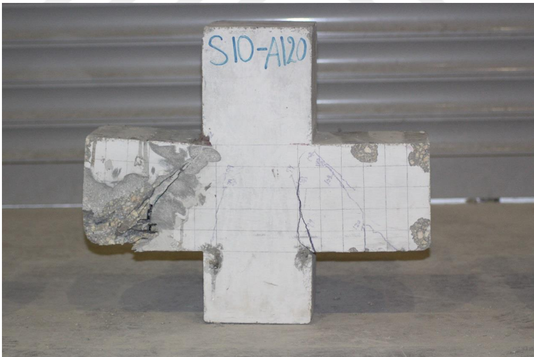
Figure 4.56 Unconfined (Specimen S10 - A120) after testing
