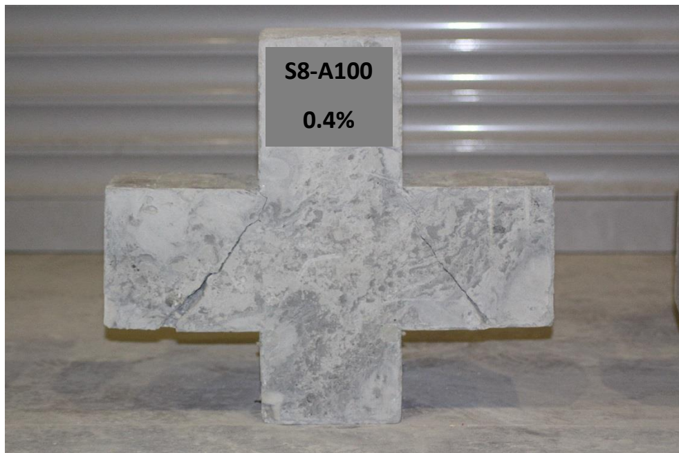
Figure 4.20 Unconfined (Specimen S8 - A100 - 0.4%) after testing
