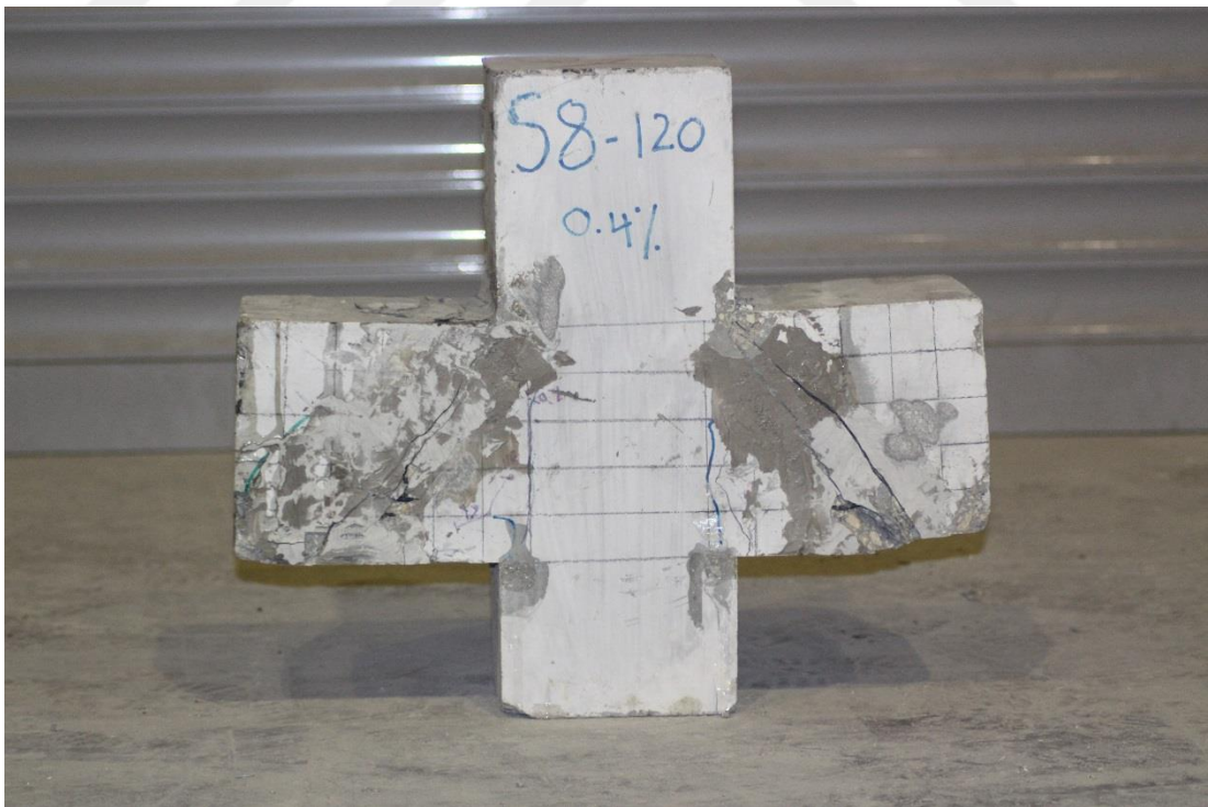
Figure 4.32 Unconfined (Specimen S8 - 120 - 0.4%) after testing
