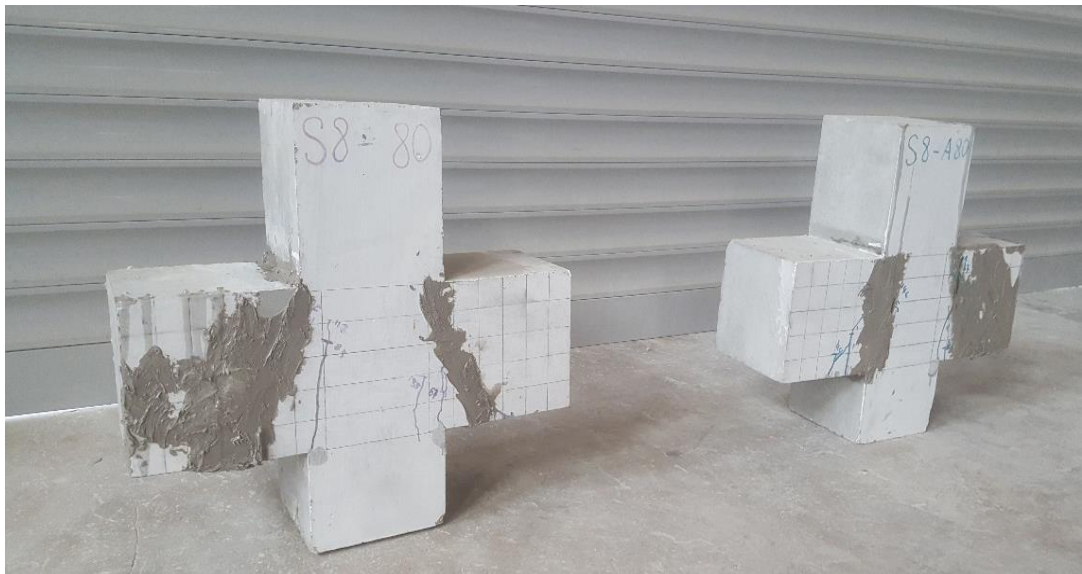
Figure 3.6 High Viscosity Epoxy coated corbels
