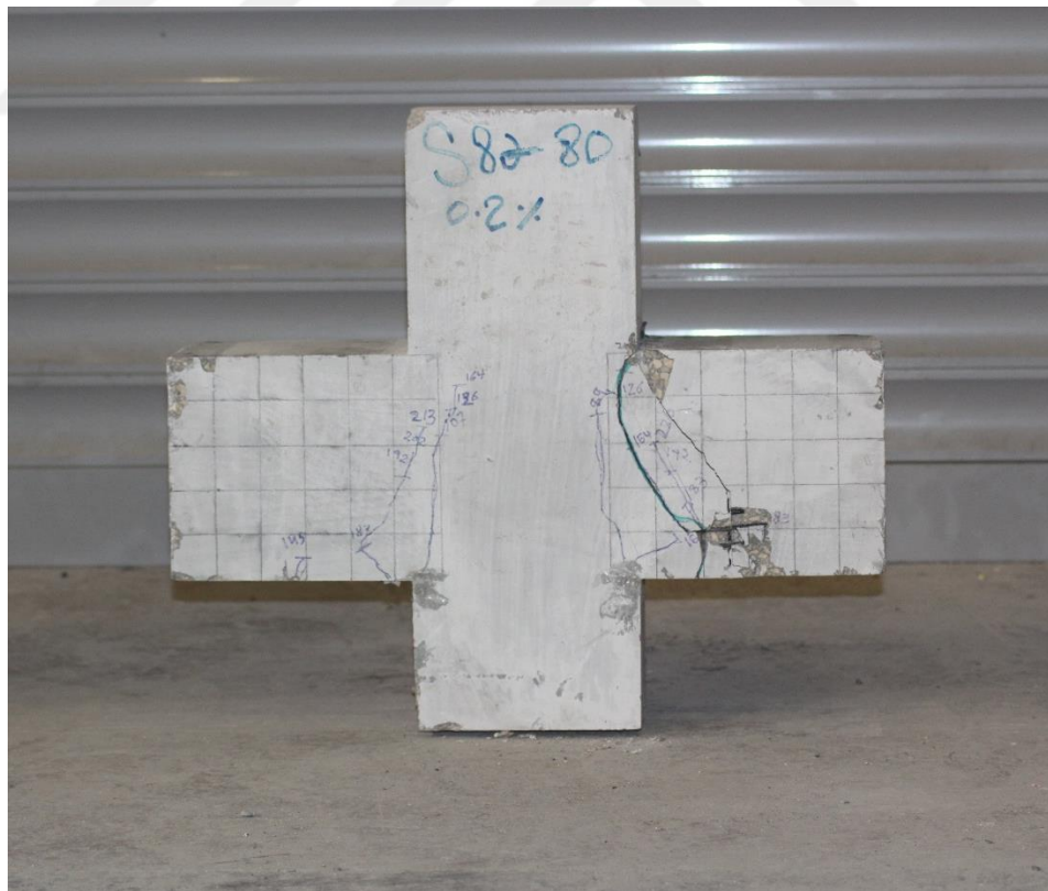
Figure 4.23 Unconfined (Specimen S8 - 80 - 0.2%) after testing
