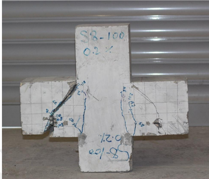
Figure 4.4 Unconfined (specimen S8 - 100 - 0.2%) after testing
