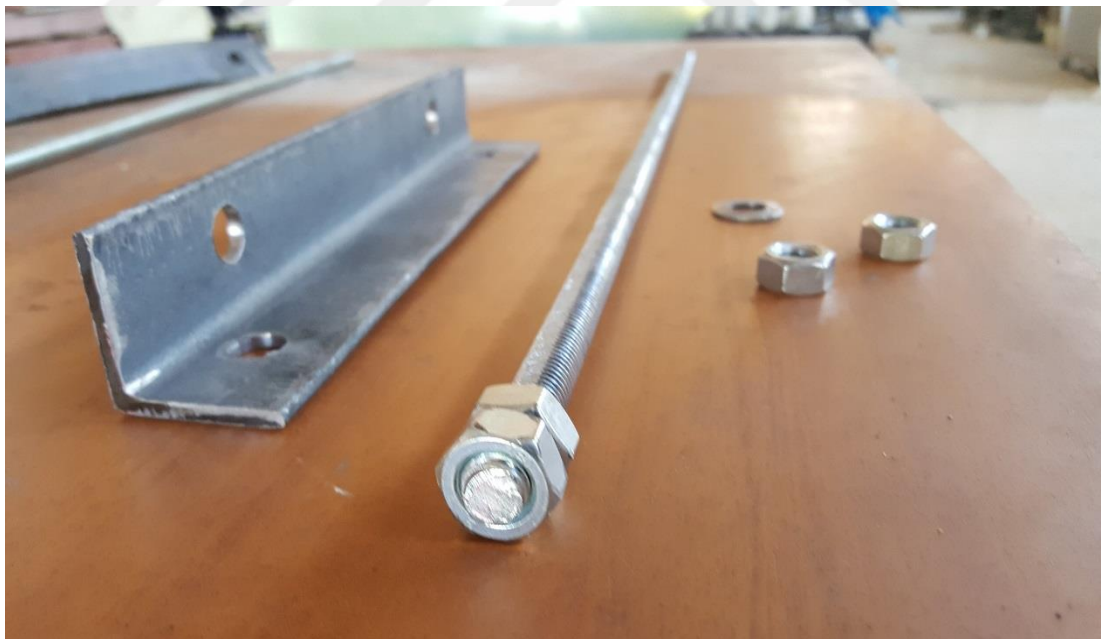
Figure 3.2 Steel Confining Elements
