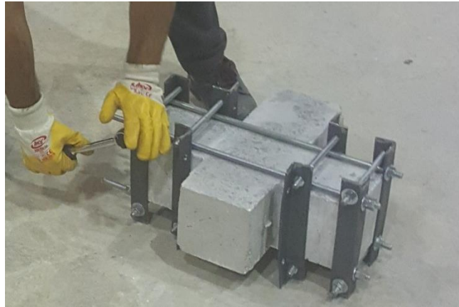
Figure 3.11 Installing the steel confinement
