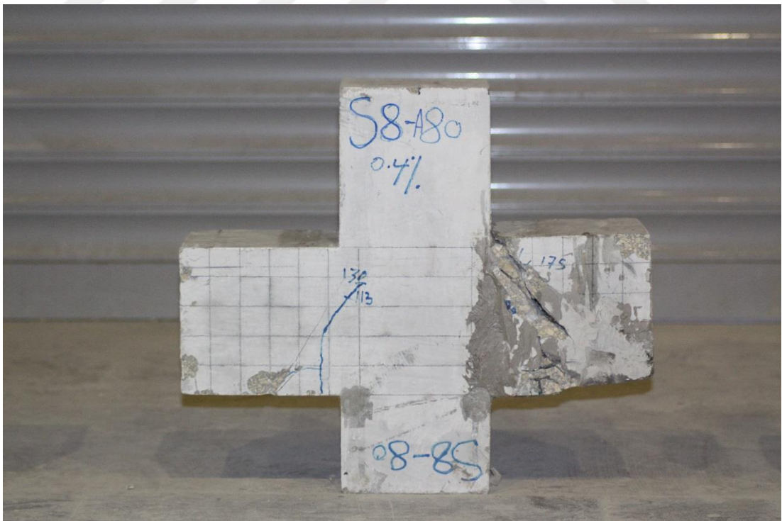
Figure 4.47 Unconfined (Specimen S8 – A80 – 0.4%) after testing
