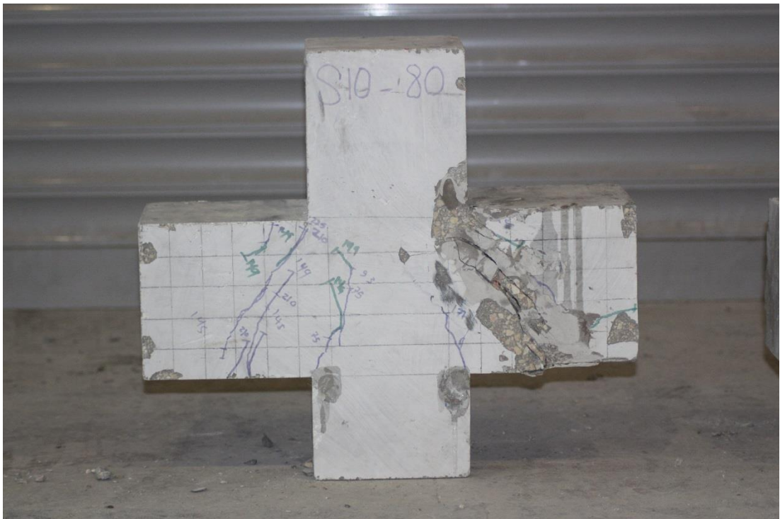
Figure 4.11 Unconfined (Specimen S10 - 80) after testing
