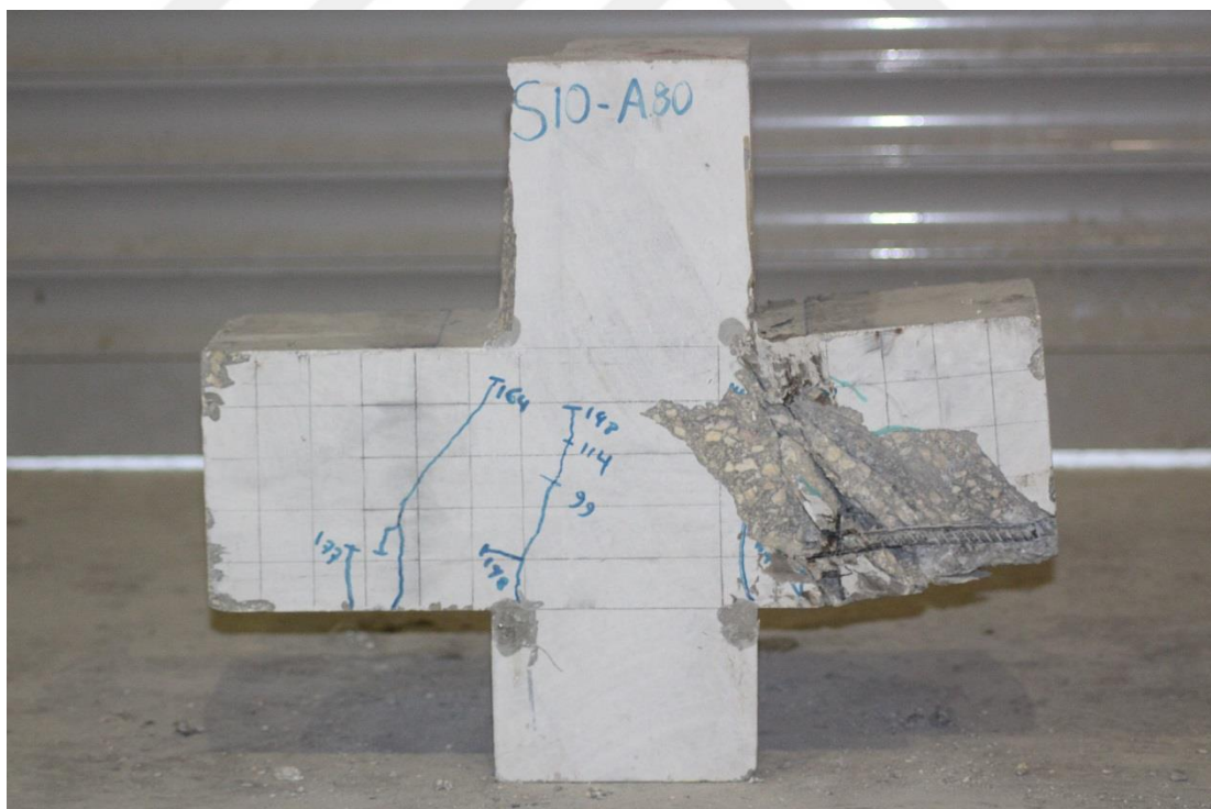
Figure 4.59 Unconfined (Specimen S10 – A80) after testing
