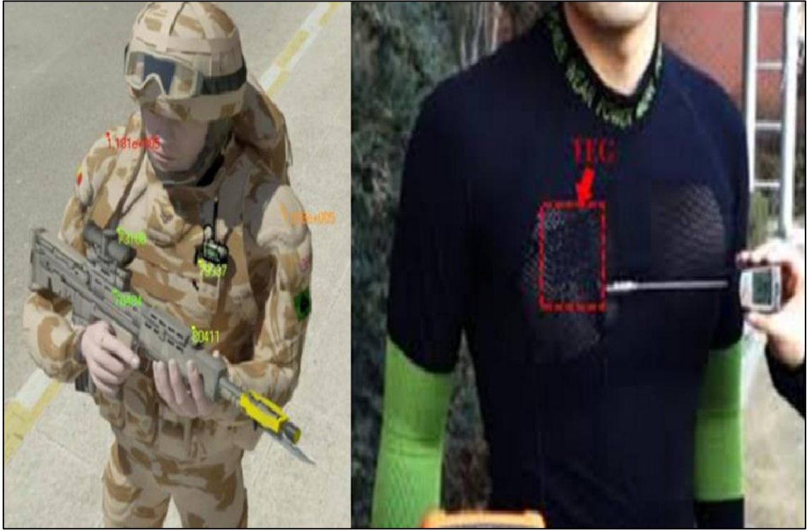
Şekil 1.13. TEG giysisi ( http://www.ecouterre.com/u-k-military-developing-solar-powered-uniforms-that-generate-electricity/ ; Kim vd., 2014).
