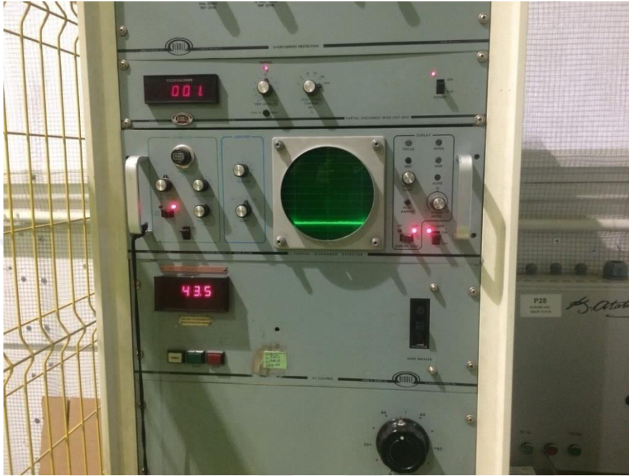
Figure 2-3 Partial discharge test equipment (Biddle 666035-01)
