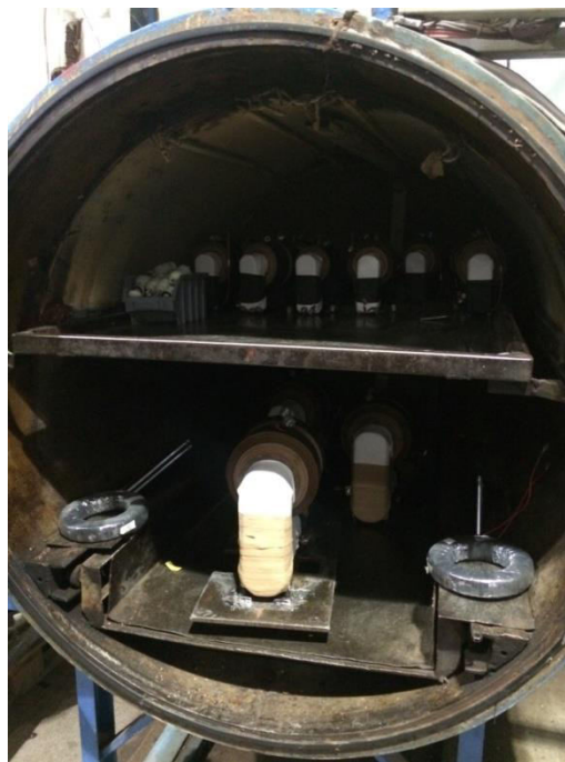
Figure 2-6 Transformer coils under heat treatment
