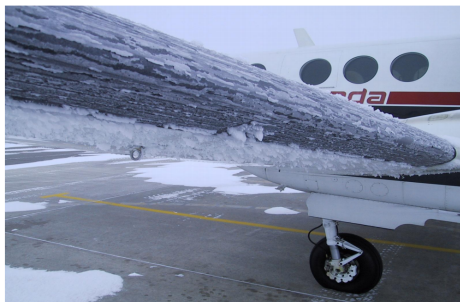
(a) Icing on aircraft wing before take-off.
