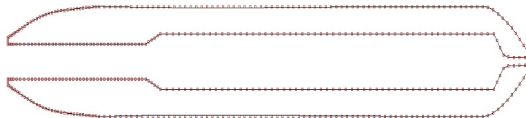
Figure 7.1: Simplified axisymmetric probe geometry used in computations.
