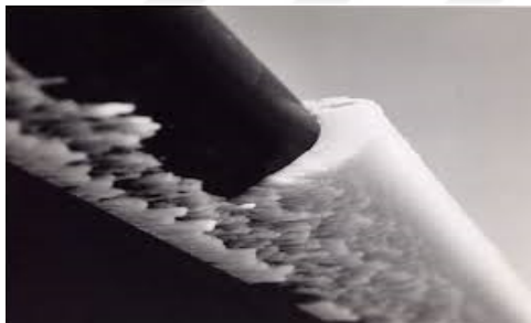
(a) Rime ice accretion on aircraft wing.
