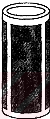
Figure 2.7: Tube piezo used in 3-dimensional sample scanner
