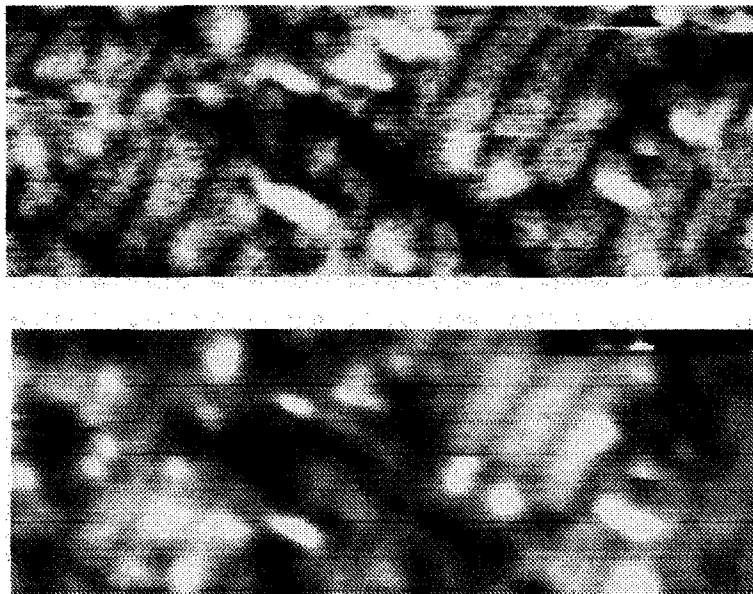
Figure 4.4: Simultaneous STM(top) and force gradient(bottom) images of Si(100) ( 2 \times 1 ) - Image size is 110 \times 38 \text{ \AA}^2 . V_{bias} = -1.5 \text{ V} , I_t = 0.5 \text{ nA} , k_o = 157 \text{ N/m} and A_o = 2.4 \text{ \AA} . Black shows more negative value in the force gradient image.
