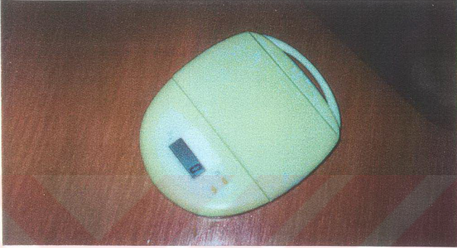
Figure 4.4. Electric balance with the accuracy of 1/1000 in (g)
