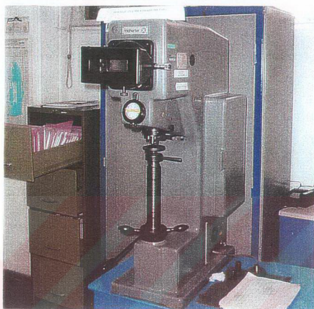
Figure 4.15. Surface hardness measuring equipment
