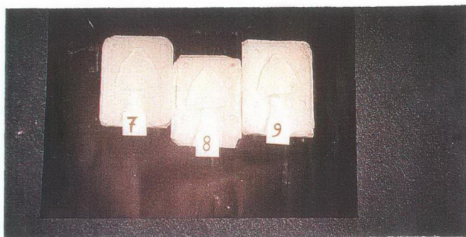
Figure 4.13. Casting molds No.7-9 for the front engine cover
