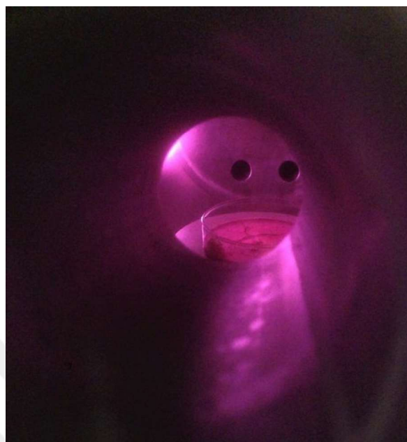
Fig. 3-17. Plasma discharge during the MWFD at 2.0 \text{ W g}^{-1} . The foam sample contained 5% (w/w) PP, 30% (w/w) MD, and 2.5% (w/w) P and was subjected to drying at a 0.1-mbar chamber pressure and 30^\circ\text{C} maximum product temperature.
