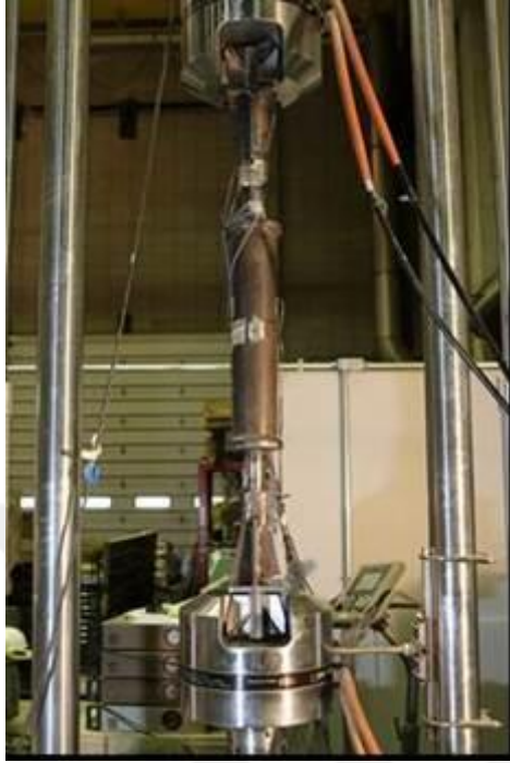
(a) Out-of-Plane Buckling
