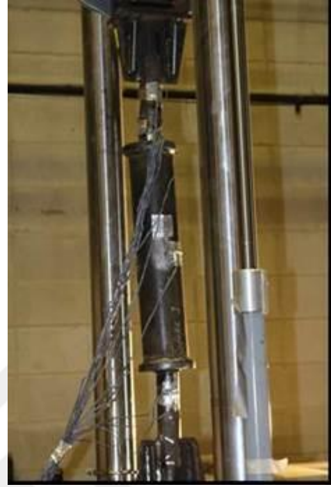
(b) In-Plane Buckling
