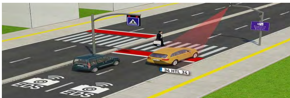
Figure 2.12 Pedestrian Crossing (Electronic Control System)
