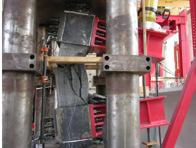
Figure 4-15 – Failure Mode of 18EB4
