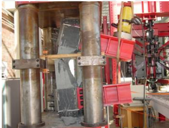
Figure 4-1 – Failure Mode of 10EB1
