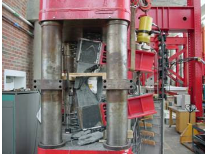
Figure 4-3 – Failure Mode of 10EB3
