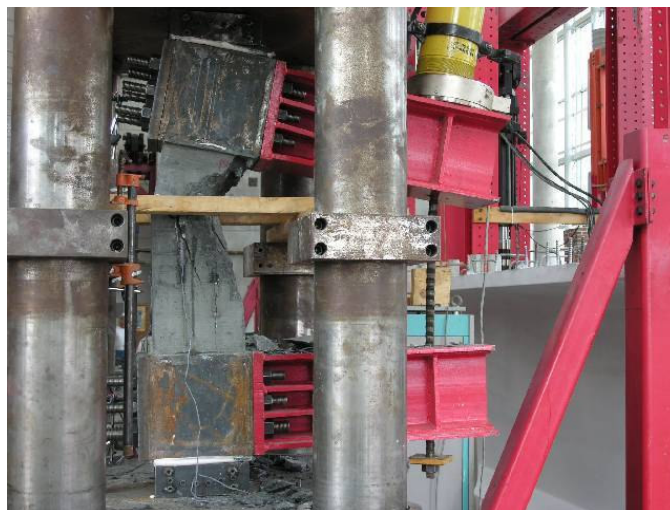
Figure 4-14 – Failure Mode of 18EB3
