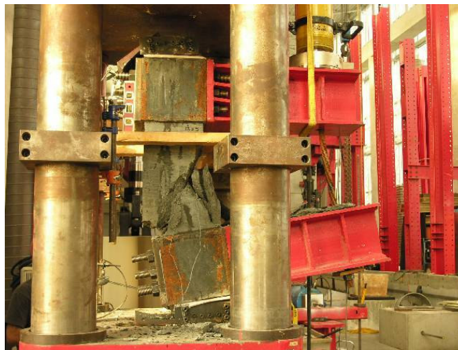
Figure 4-20 – Failure Mode of 18EB9
