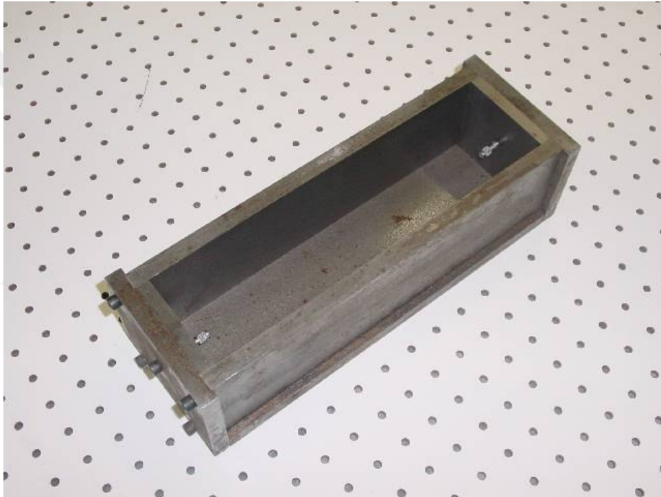
Figure 3-32 – Steel Mold for Prismatic Shrinkage Specimens
