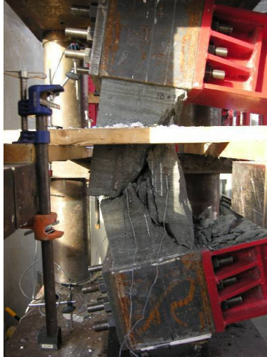
Figure 4-18 – Failure Mode of 18EB7
