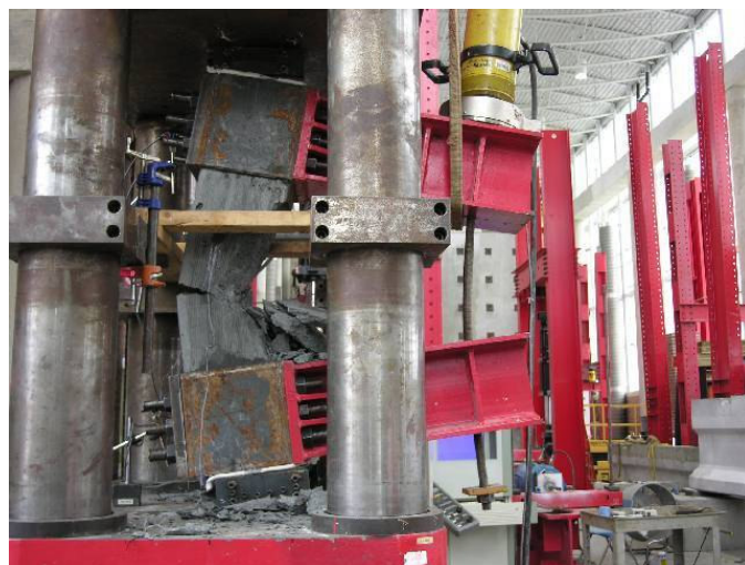
Figure 4-5 – Failure Mode of 10EB5
