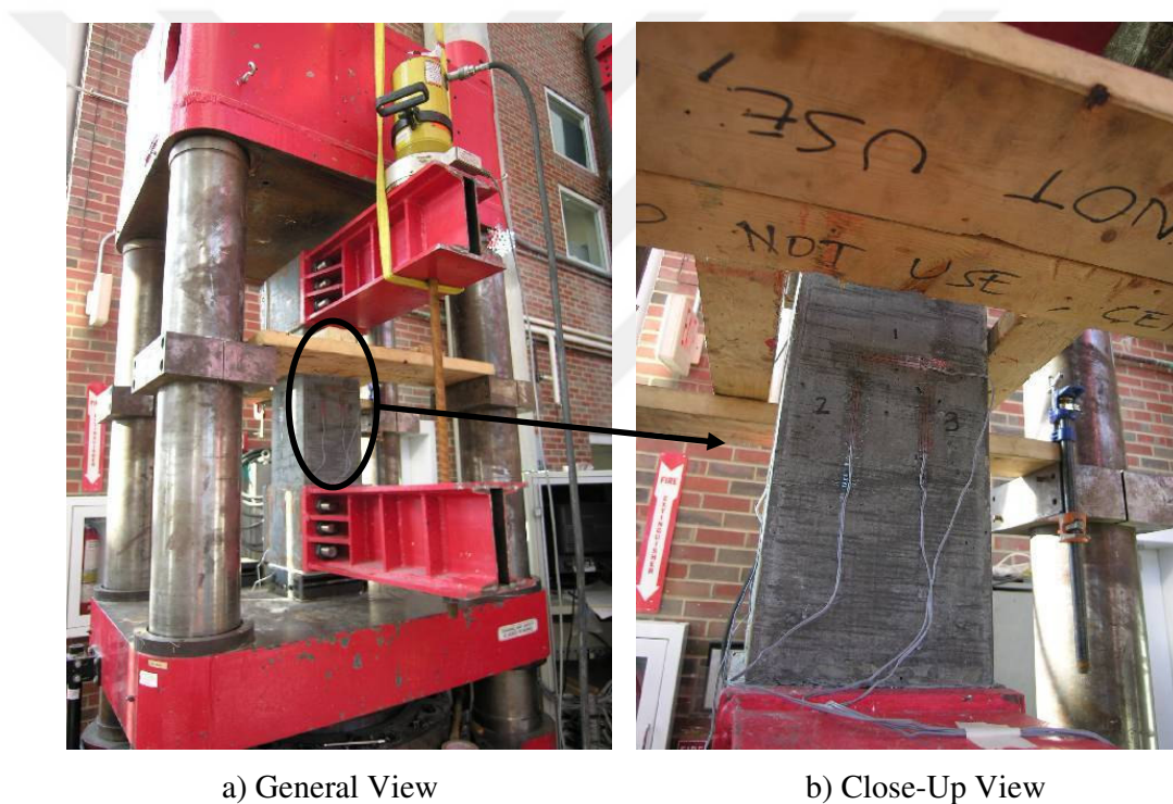
Figure 4-27 – Compression Face of Eccentric Bracket Specimen
