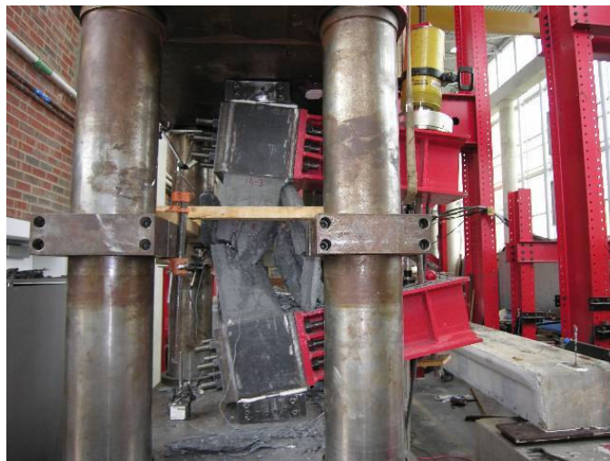
Figure 4-8 – Failure Mode of 14EB3
