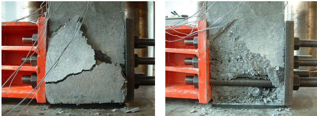
Figure 3-3 – Failure Mode at the Lower End of Pilot Specimen 1
