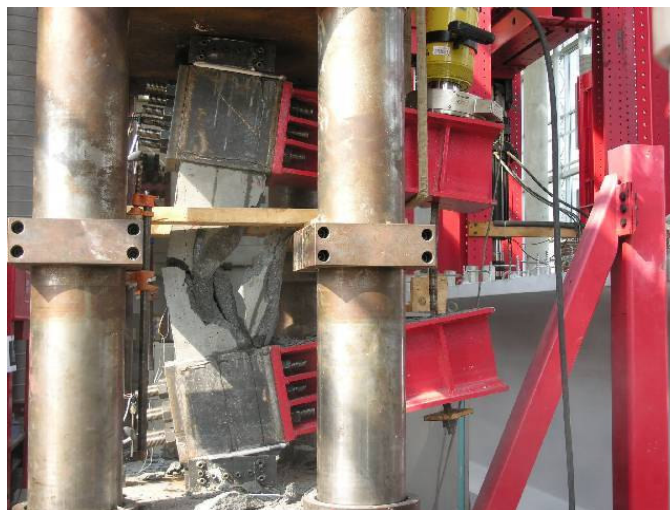
Figure 4-17 – Failure Mode of 18EB6
