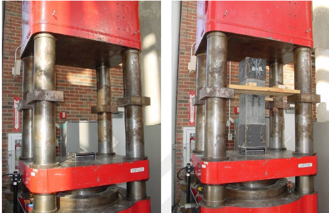
Figure 3-16 – Placement of the Specimen into the Compression Machine
