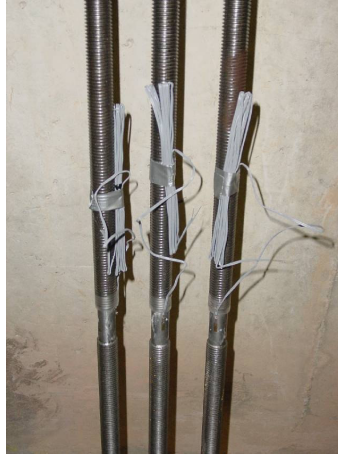
Figure 3-23 – Application of the Strain Gages
