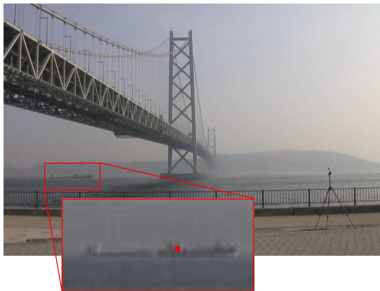
Figure.5.5 Tracking point of ship in image sequences
