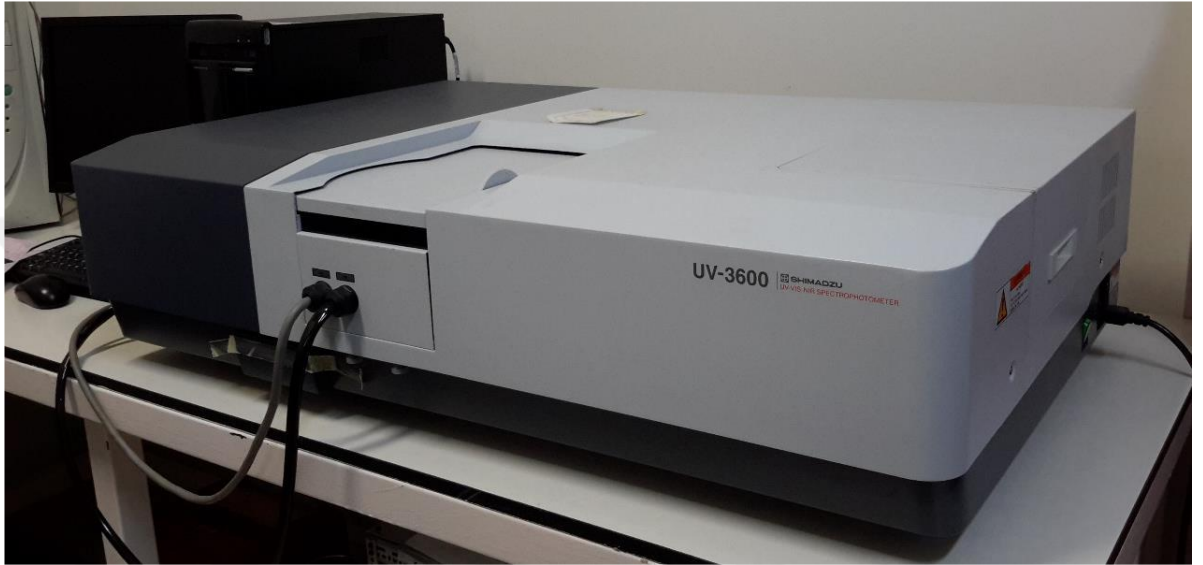
Figure 3.2 Shimadzu 3600 UV-Vis-NIR spectrophotometer [137].
