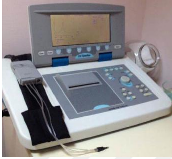
Şekil 2.7: GSI (Grason – Stader Inc.) Tymptstar middle ear analyzer version 2
