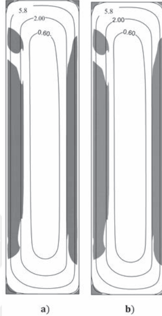
Figure 2.3: Contours of non-dimensional stream function \Psi with unyielded regions (i.e. grey regions) for AR = 4 for differentially heated from side walls configuration, a) R^\lambda = 10^{-6} , b) R^\lambda = 10^{-7} at r_i/L = 1.0 , Ra = 10^6 , Bn = 0.2 and Pr = 500 for CWHF boundary condition.
