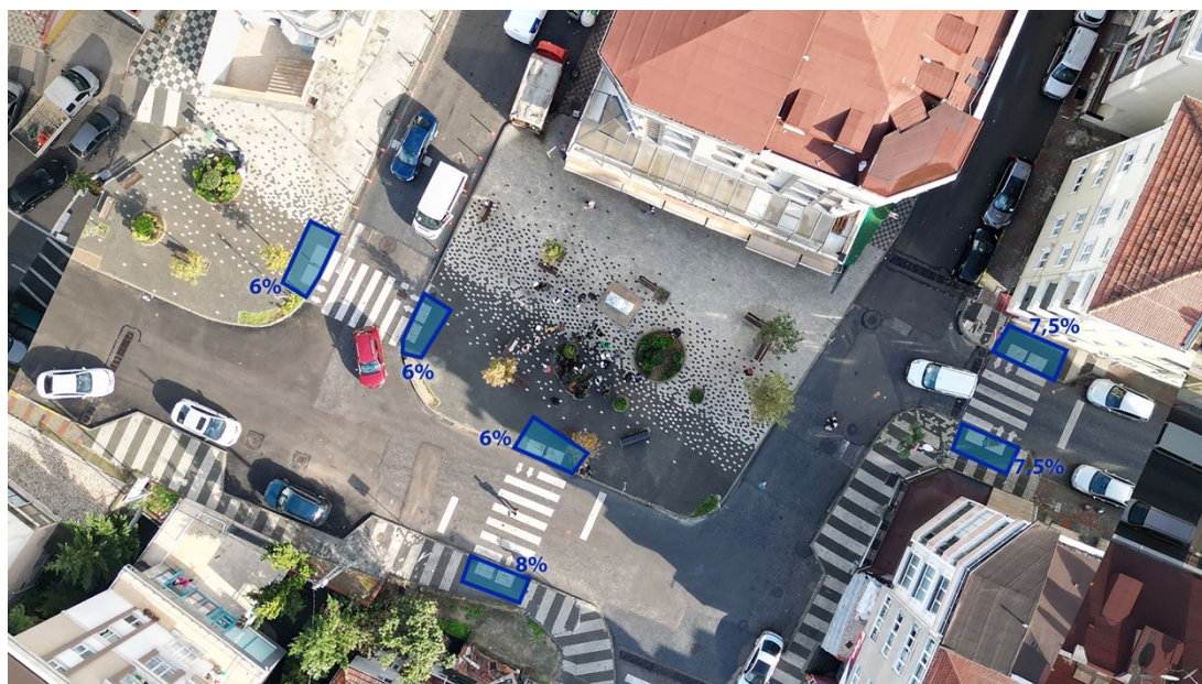
Figure 4.18 : Slope measurements of ramps (Superpool,2020)
