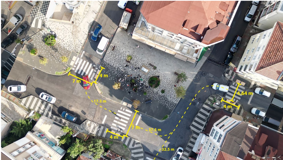
Figure 4.9 : Measurements of pedestrian crossings (Superpool,2020)
