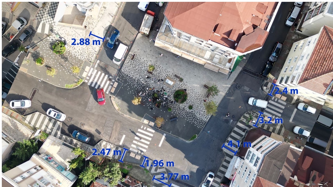
Figure 4.17 : Sidewalk widths (Superpool,2020)
