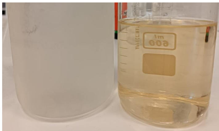
Figure 3.2 Acetone collected after the precipitation stage of a successful LevMA production (clear and transparent) and acetone collected after an unsuccessful LevMA production (orange)
