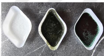
Figure 2.2. Solution poured into leaf-shaped molds for film structure
