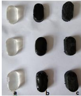
Figure 2.4 Gel samples in the form of drug tablets (a) gelatin gel (b) Spirulina + gelatin gel (c) Chlorella + gelatin gel
