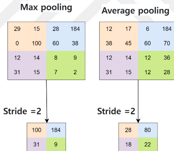
Figure 3.4. Illustrate how 2D max pooling and avg pooling work, with the following setting: kernel size [2, 2], stride [2, 2].
