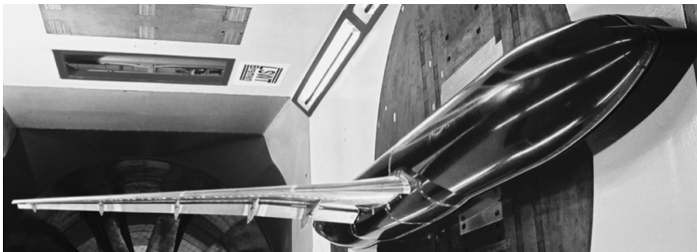
Figure 1.16 : DLR-F11 in the B-LWST Wind Tunnel, AIAA 2nd High Lift Prediction Workshop [7]
