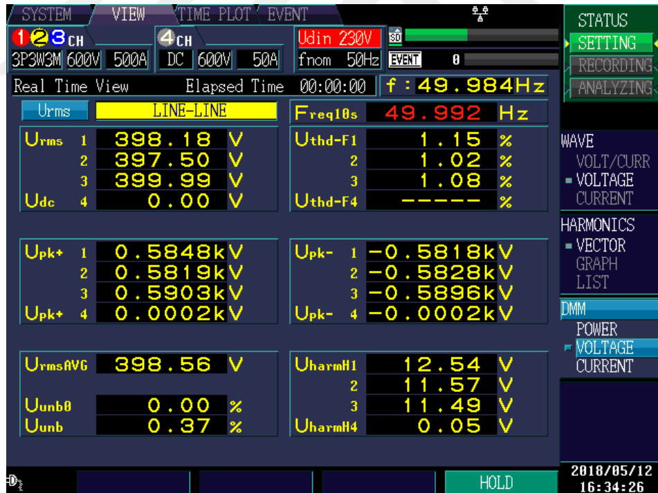
Figure 4-42 Input line-to-line voltages and their THD values
