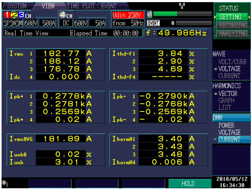
Figure 4-43 Input line currents and their THD values
