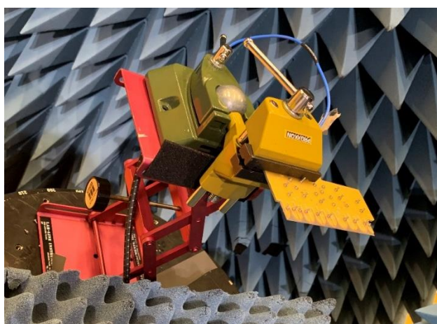
Figure 4.35. 8x1 Vivaldi array combined with the 8-way power divider under test.
