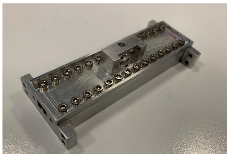
Figure 4.12. Ridged-waveguide section to mount the single probe.
