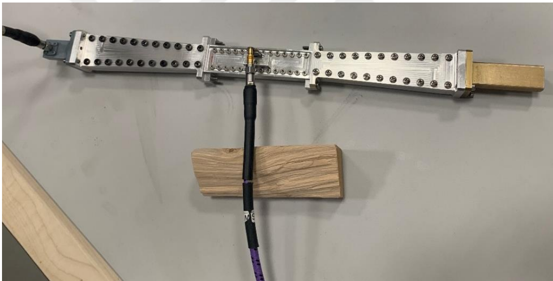
Figure 4.14. Measurement setup for the unit cell with the single probe.
