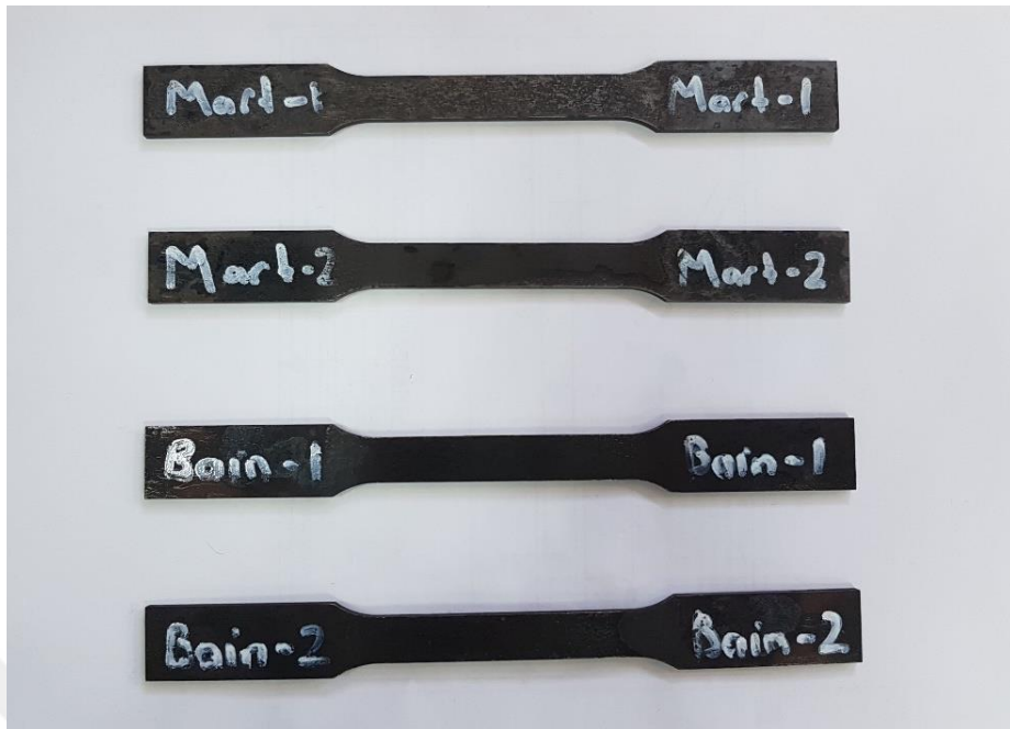
Figure 3.8. Tensile Test Specimens before Tensile Tests
