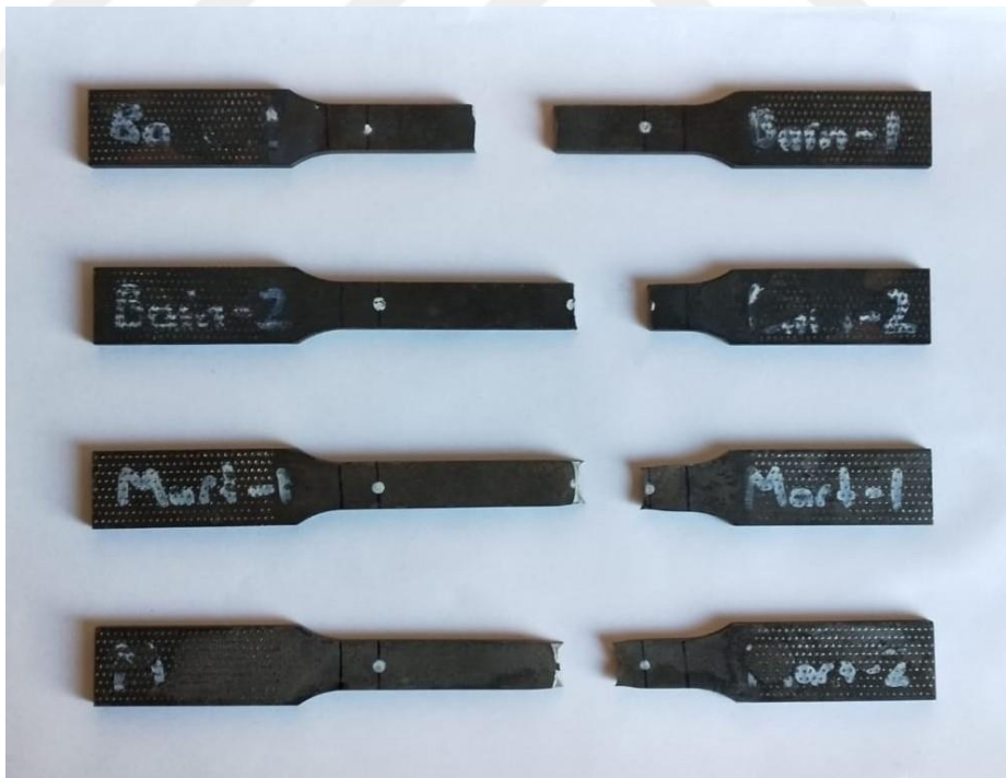
Figure 3.9. Tensile Test Specimens after Tensile Tests
