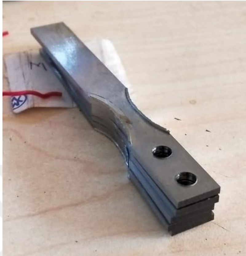
Figure 3.33. Fatigue Specimens after CNC Machining Operation
