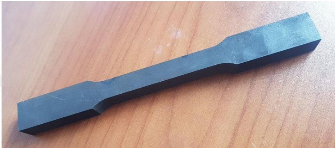
Figure 3.5. A Semi-Product Tensile Test Specimen
