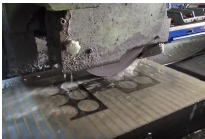
Figure 3.28. Fatigue Specimens during First Grinding Operation
