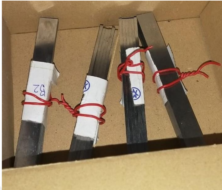
Figure 3.29. Fatigue Specimens after First Grinding Operation
