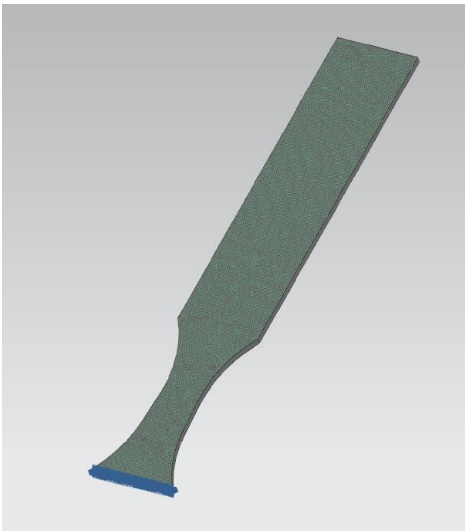
Figure 3.20. Application of Constraint on Meshed Fatigue Specimen Model for Numerical Modal Analysis
