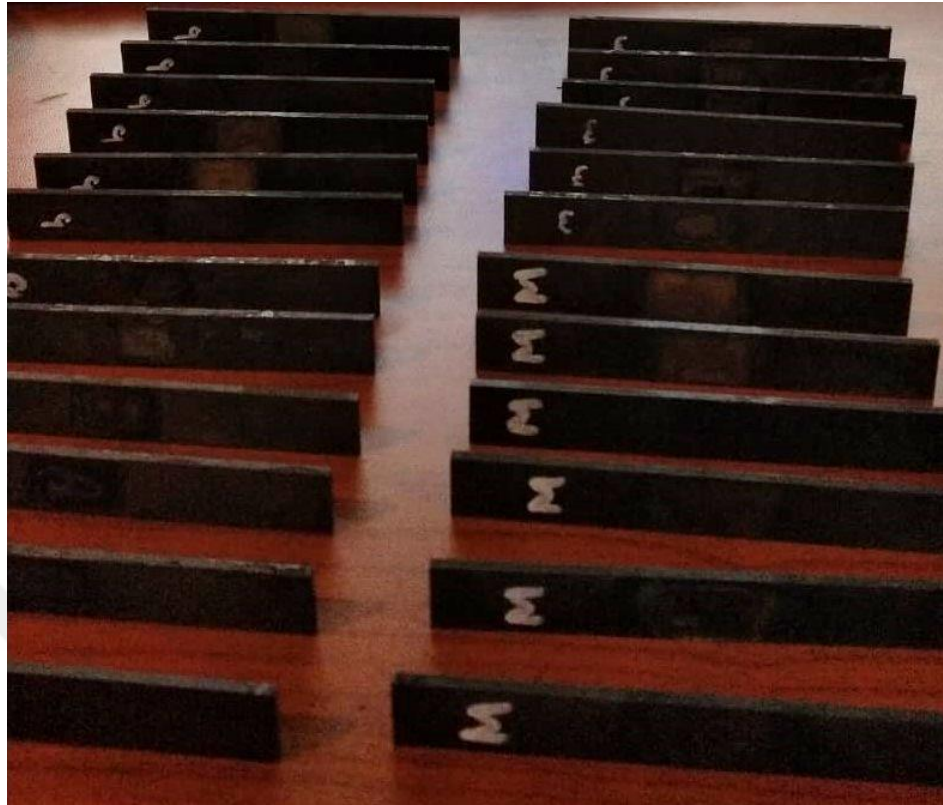
Figure 3.26. Fatigue Specimens after Heat Treatment Processes
