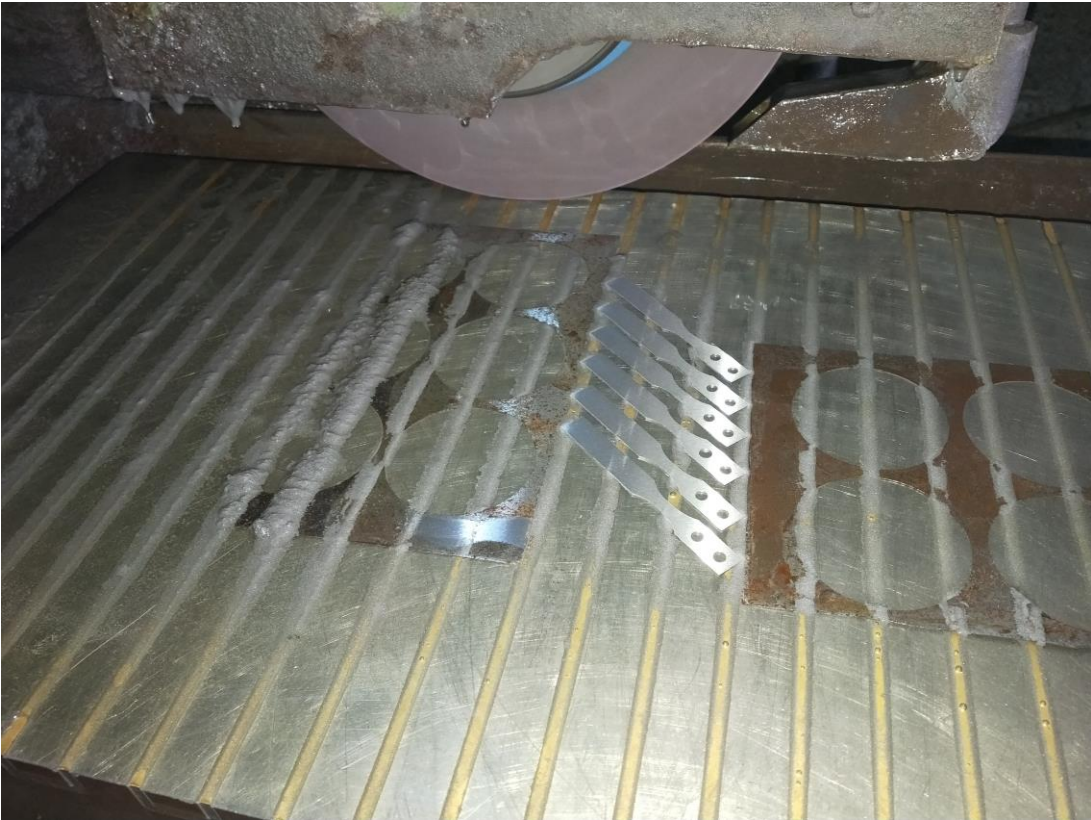
Figure 3.36. Fatigue Specimens during Finish Grinding Operation
