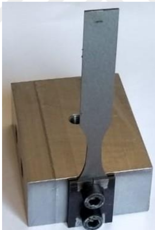
Figure 3.43. Fixation of Fatigue Specimen to Fatigue Test Machine
