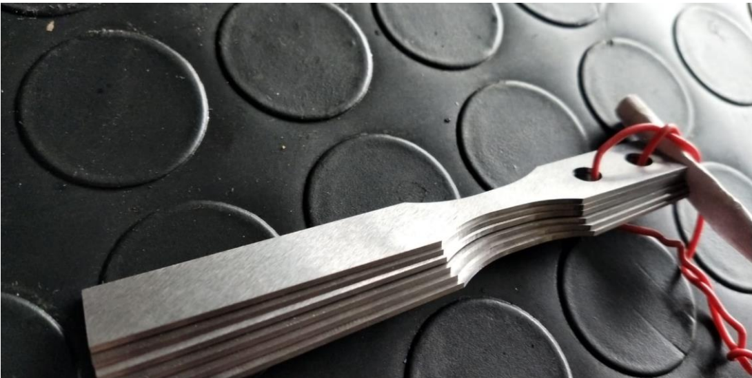
Figure 3.37. Finished Fatigue Specimens
