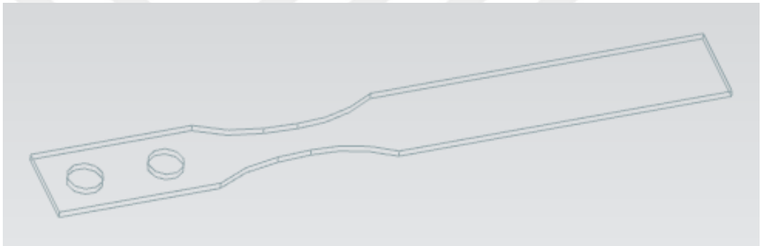
Figure 2.11. Hybride Model of Bell Telephone Laboratories Type and Krouse-type Fatigue Specimen
