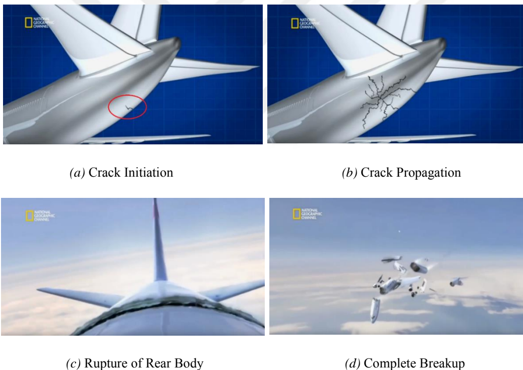
Figure 1.2. Illustration [by Nat Geo TM ] of Fatigue Failure of the Aircraft which belonged to China Airlines Flight 611
