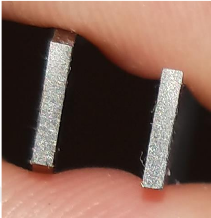
Figure 4.31. Fracture Surfaces of a LB-250 Fatigue Specimen
