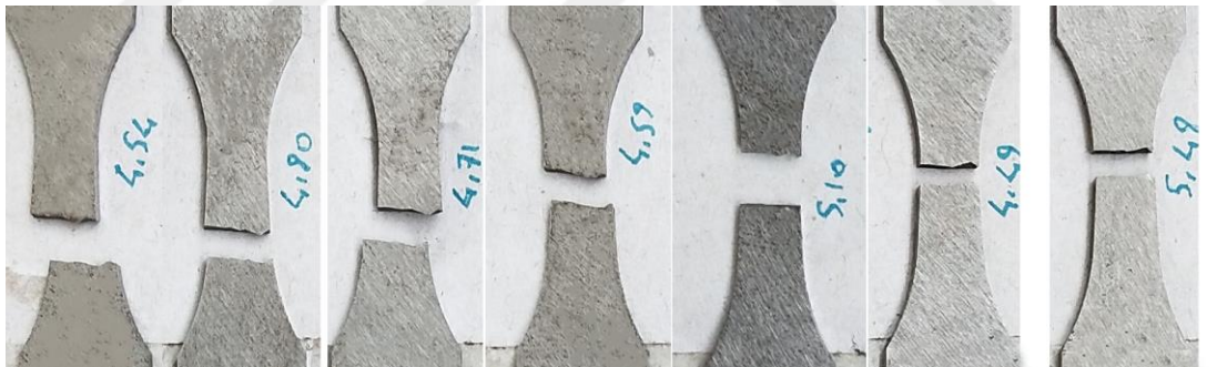
Figure 4.34. Fracture Zones of TM-400 Fatigue Specimens
