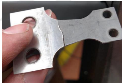
Figure 2.7. A 316L Krouse-type Fatigue Specimen with Characteristic Crack just before Final Fracture [17]
