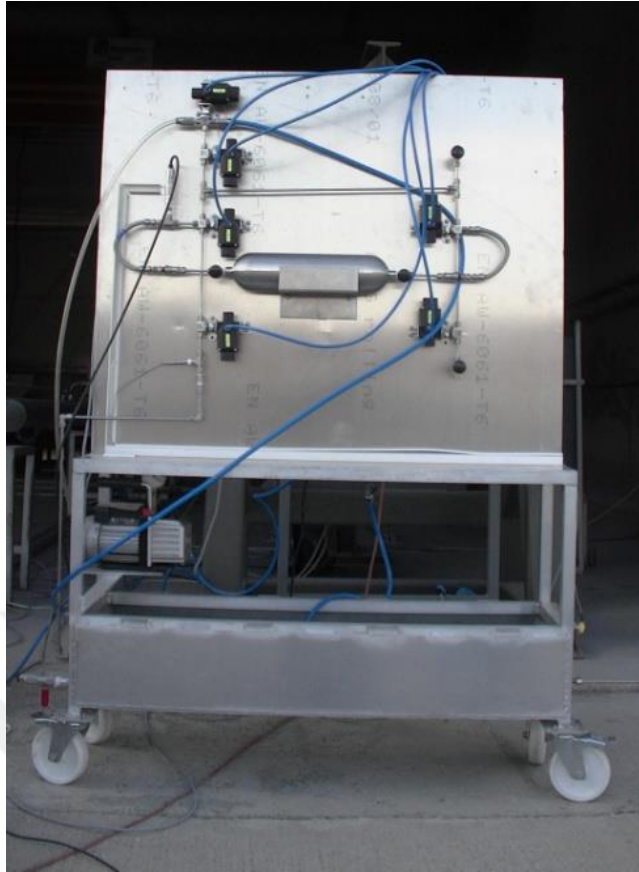
Figure 4.17: Gas sampling system with the sampling tube.
