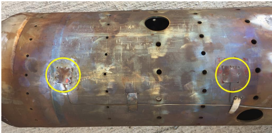
Figure 4.21: Surface thermocouples on the CAH liner.
