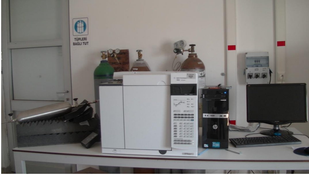
Figure 4.19: Gas chromatography device.
