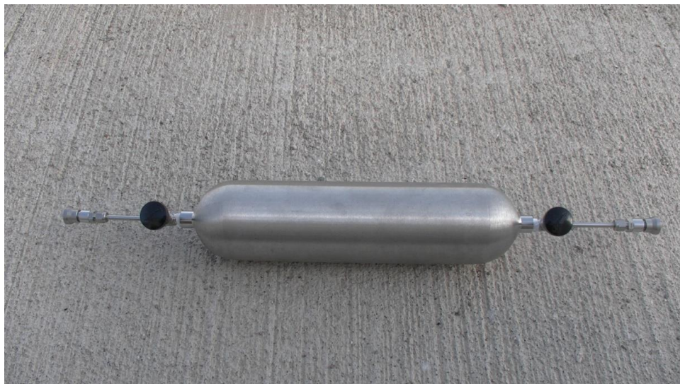
Figure 4.16: Gas sampling tube.
