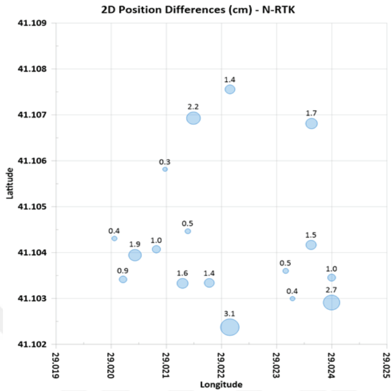
Figure A.1 : Horizontal differences between static GNSS and N-RTK model outputs
