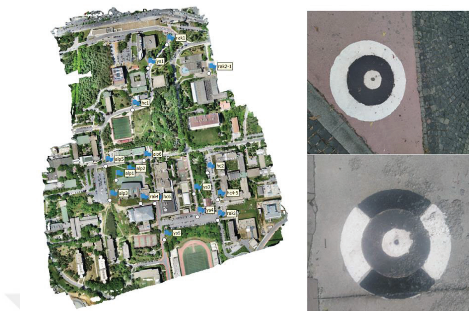
Figure 4.3 : GCPs locations (left) and painted ground control points (right)
