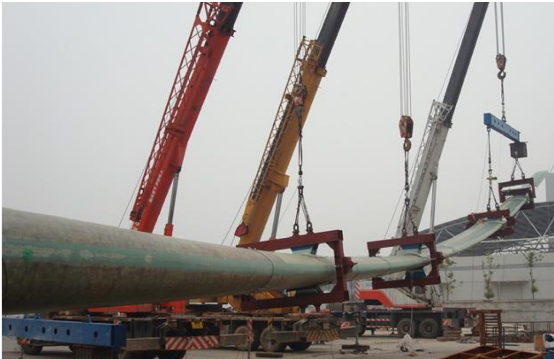
Figure 2.10. A full-scale wind turbine blade under flap-wise loading static test [21]
