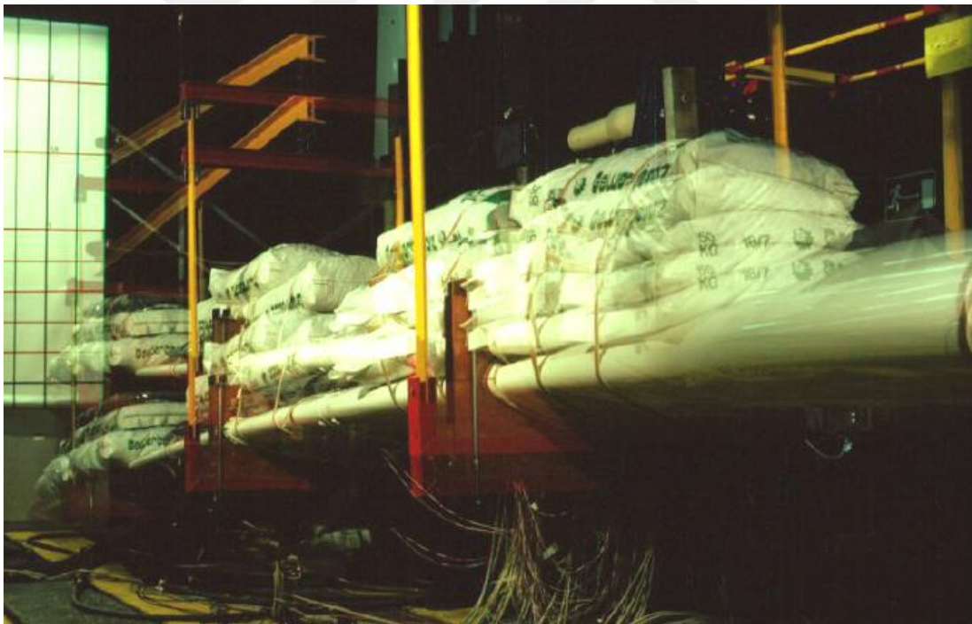
Figure 1.6. Distributed Surface Loads [14]
