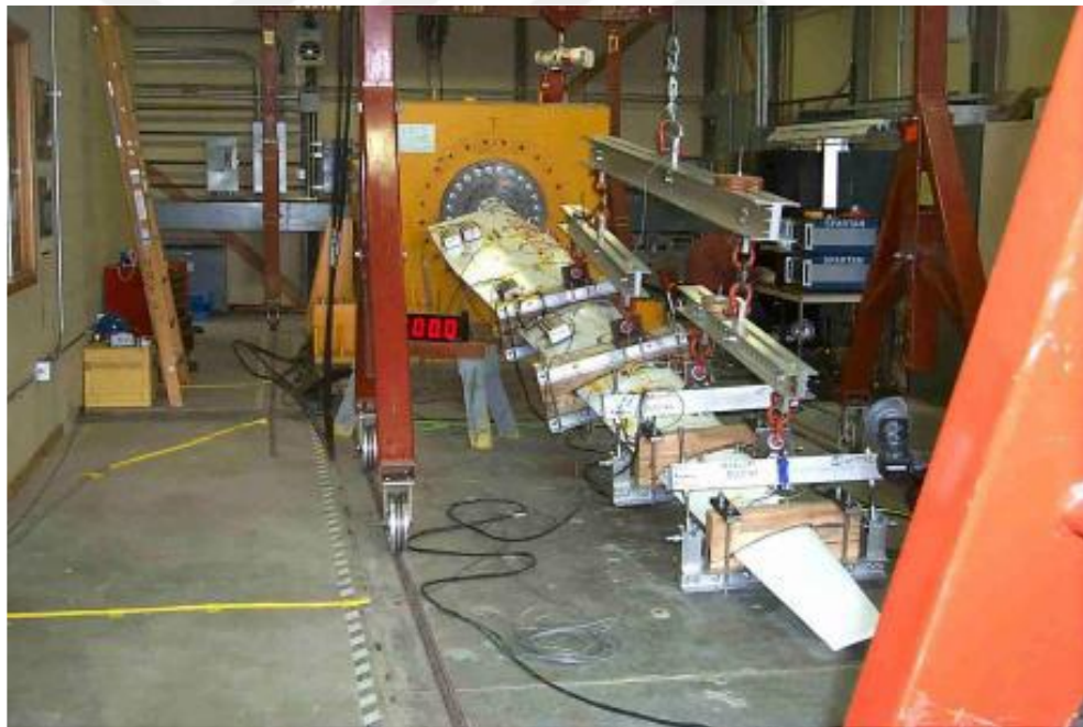
Figure 2.9. Whiffletree arrangement on 9 meters wind turbine blade [20]
