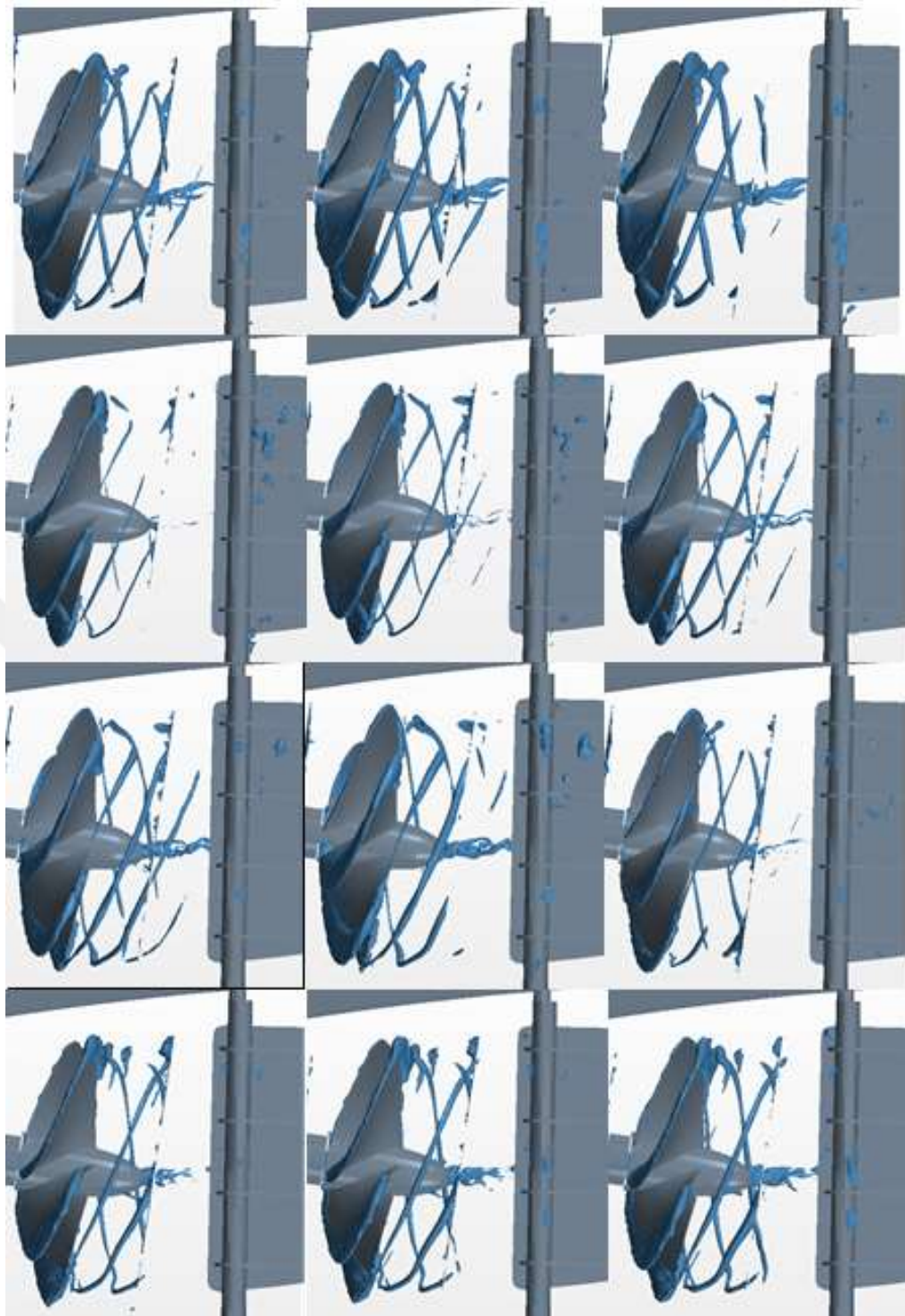
Figure 7-19 CFD Results - Cavitation Patterns including tip vortex cavitation (Model Scale)
