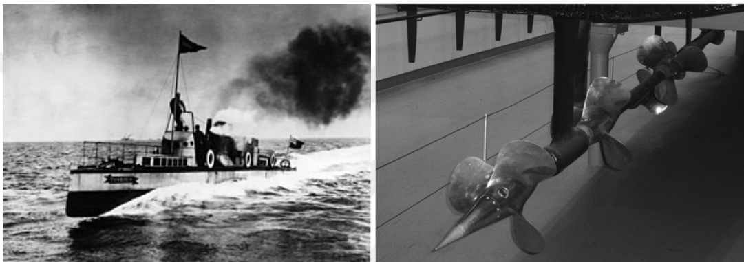
Figure 2-1 Turbinia and its triple propeller arrangement on a shaft line
