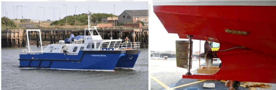
Figure 3-9 Left: Deep-V Hull Form Catamaran ‘Princess Royal’, Right: Princess Royal Propeller
