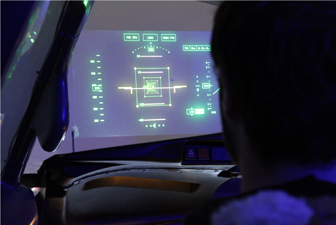
Figure 3.5: Transparent Screen overlay for HUD augmented reality implementations. pilot effective flight direction perception. The brief descriptions of the nominal HUD symbols can be seen in Figure 3.6.
