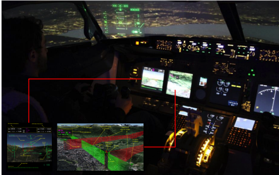
Figure 3.1: B737 – 800 Flight Deck test platform in ITU CAL with experimental visual decision support tools for future ATM realm: Head up Display (HUD), Synthetic Vision Display (SVD) and 4D Operational Display (4DOD).
