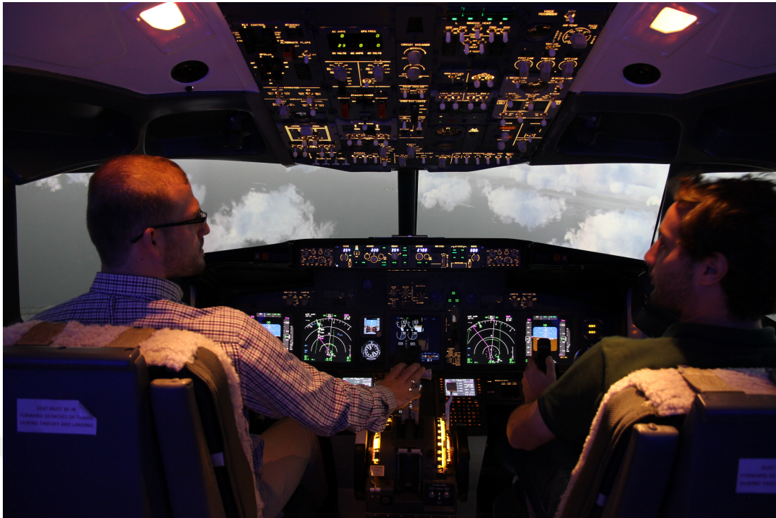
Figure 2.2: Boeing 737-800 full replica flight deck testbed of ITU Aeronautics Research Center in a nominal tactical operation.
