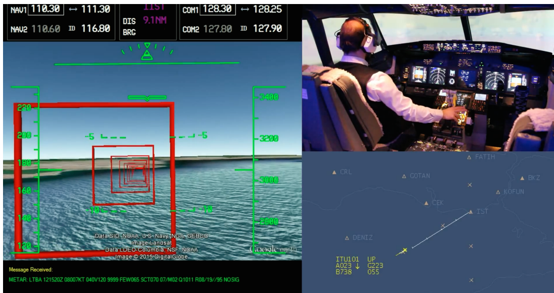
Figure 2.10: Radar screen of the controller and synthetic vision screen of the pilot during co-simulation for landing scenario.
