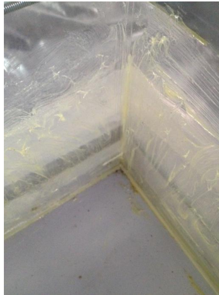
Figure 7.3. Gres oil application on the sides of the soil box.
