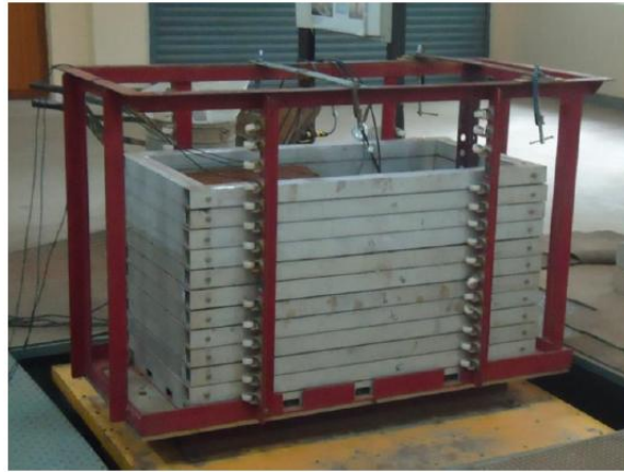
Figure 6.5. Laminar box used for the experiments (Srilatha et al. , 2012).
