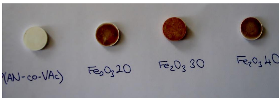
Figure 3.4 : Pellets of precipitated with EtOH and dried P (AN-co-VAc), P(AN-co-VAc)/Fe 2 O 3 (20), P (AN-co-VAc)/Fe 2 O 3 (30), P (AN-co-VAc)/Fe 2 O 3 (40) powders after polymerization.
