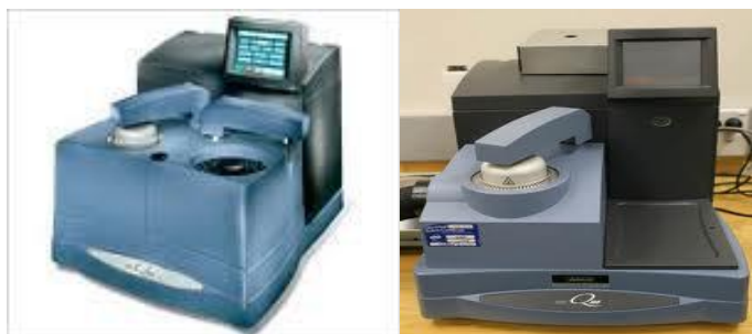
Figure 3.12 : TA Q 1000 DSC on the left, Perkin Elmer Q 600 TGA on the right.
