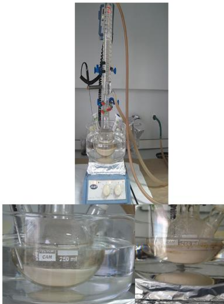
Figure 3.3 : Experimental setup for synthesis of P (AN-co-VAc)/Fe 2 O 3 .
