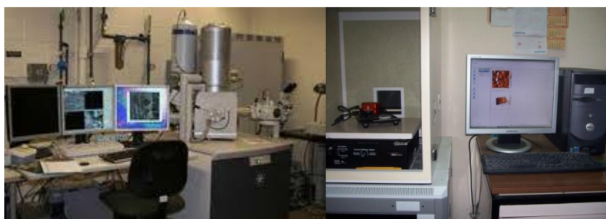
Figure 3.11 : Scanning Electron Microscope (FEI - Quanta FEG 250) on the left, Atomic Force Microscope (Nanosurf EasyScan2 STM) on the right.
