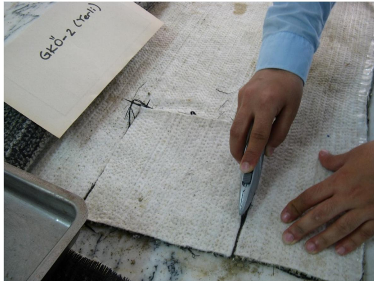
Figure 1. Cutting square GCL
