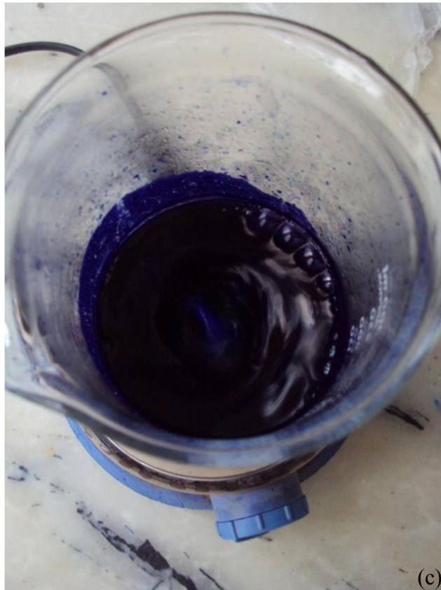
Figure 4. b), c) Mix the bentonite suspension (Continue)
