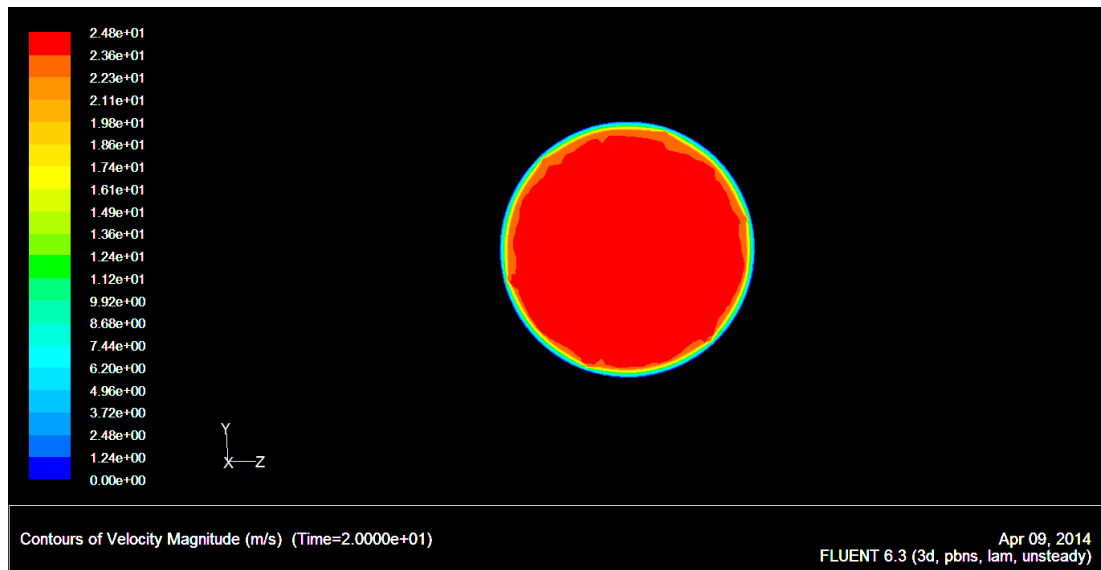
Figure 3.51. Velocity magnitude contours of the orifice area only
