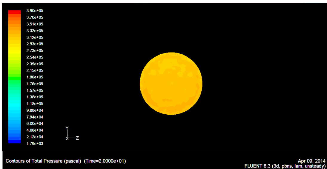
Figure 3.53. Pressure contours of the orifice area
