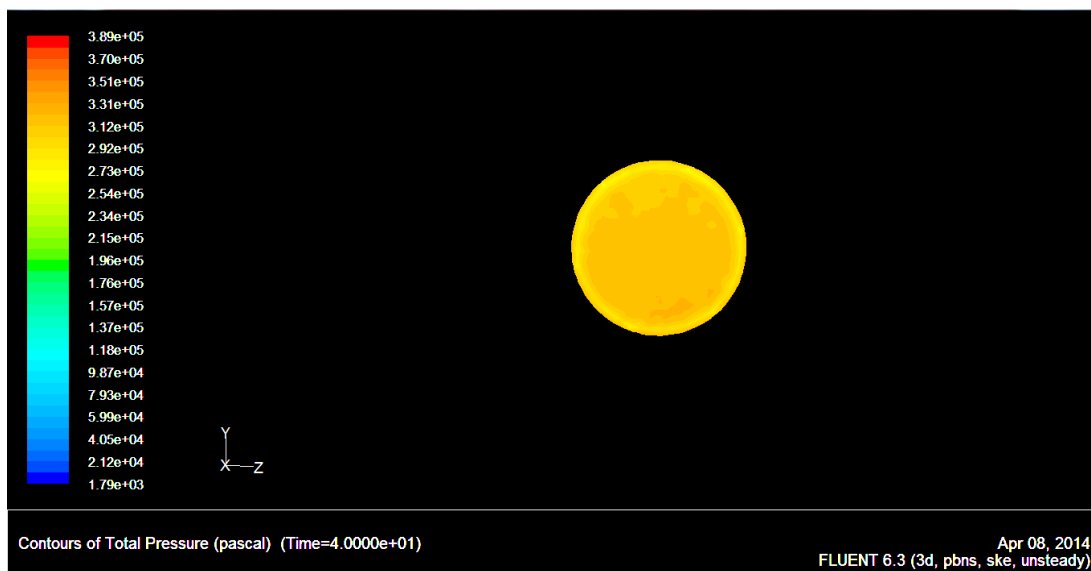
Figure 3.67. Pressure contours of the orifice area
