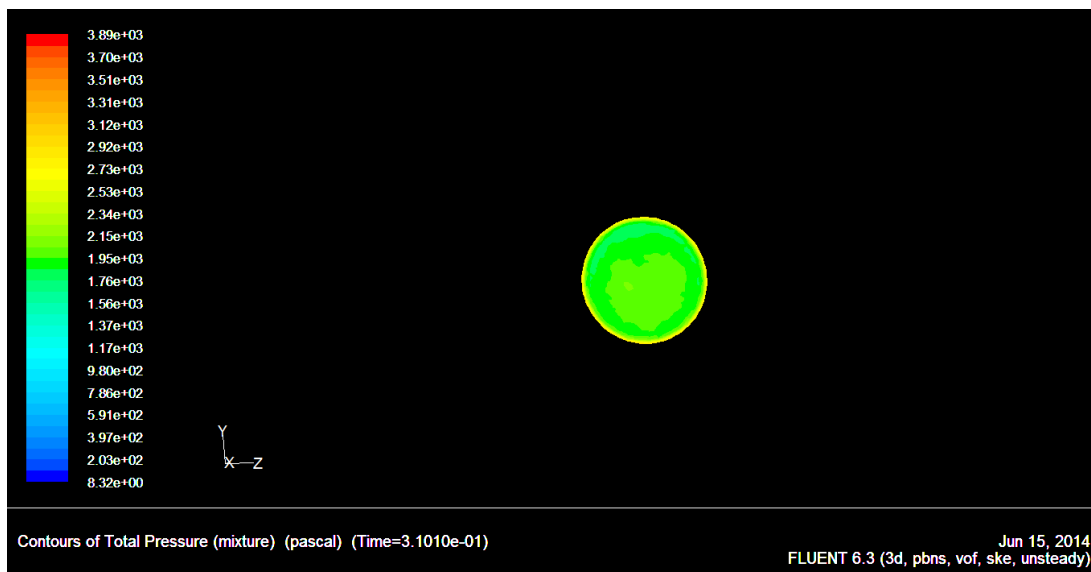
Figure C.14. Pressure contours of the orifice area
