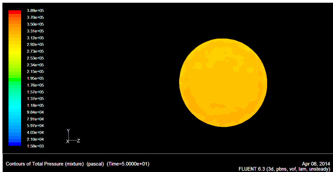
Figure 3.81. Pressure contours of the orifice area only
