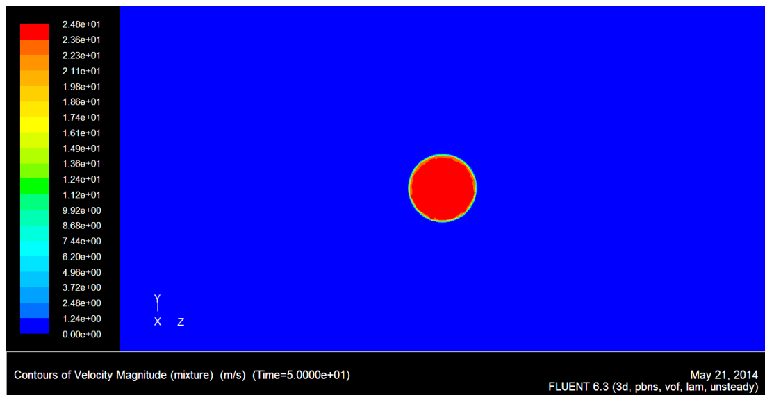
Figure 3.78. Close up of the orifice area for the contours of velocity magnitude
