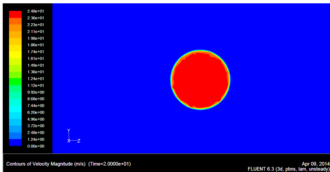
Figure 3.50. Close up of the orifice area for the contours of velocity magnitude
