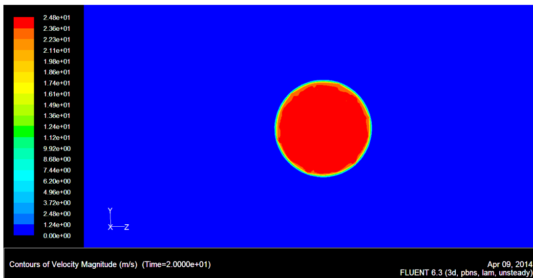
Figure 3.64. Close up of the orifice area for the contours of velocity magnitude
