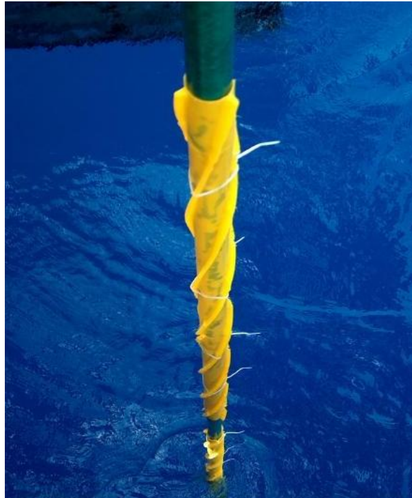
Figure 1.11. Helical strakes used around a pipe ( http://web.mit.edu/shear7/experiments.html )
