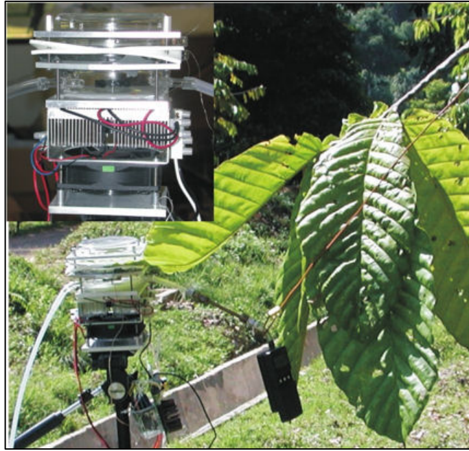
Figure 2.2 Application of a leaf cuvette system (Harley et al., 2004).
