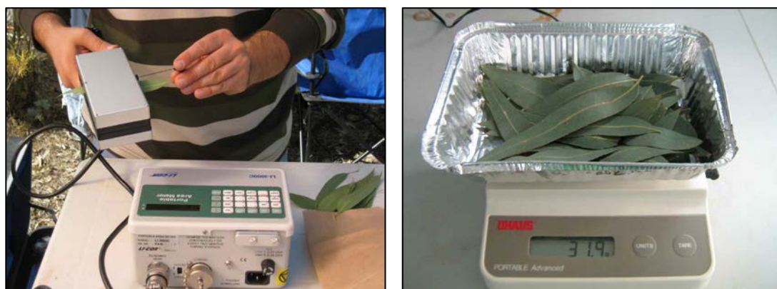
Figure 3.6 Measuring enclosed leaf area and foliage weight.
