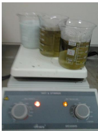
Figure 3.2 : Mixing and heating of precursors with different chealating agents on magnetic stirrer.
