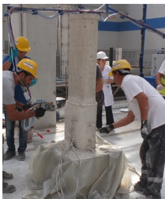
Figure 2.9: Process of column retrofitting: (a) Saturation of retrofitting region by water before retrofitting process. (b) Leaving a gap between column and stub by wooden elements. (c) Sparying GRC. (d) Wrapping Basalt textile. (e) Wrapping Basalt and sparying GRC. (f) Retrofitted Column
