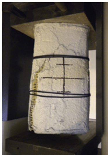
Figure 1.2: Typical failure of confined square specimen.
