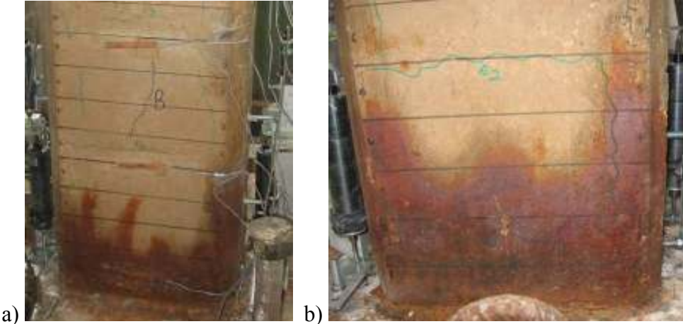
Figure 6.118 : a) North, and b) South view of the specimen LS-X19-H after -2.00% drift ratio.
