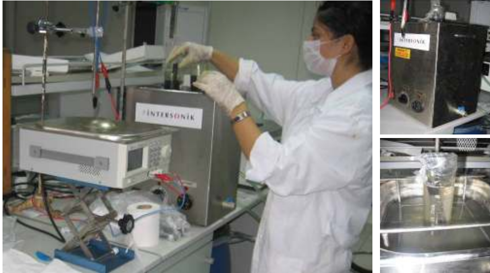
Figure 6.126 : Cleaning process of corroded reinforcement removed from reinforced concrete test specimens.
