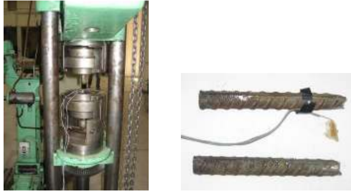
Figure 6.127 : The test setup and a fractured bar after the test.
