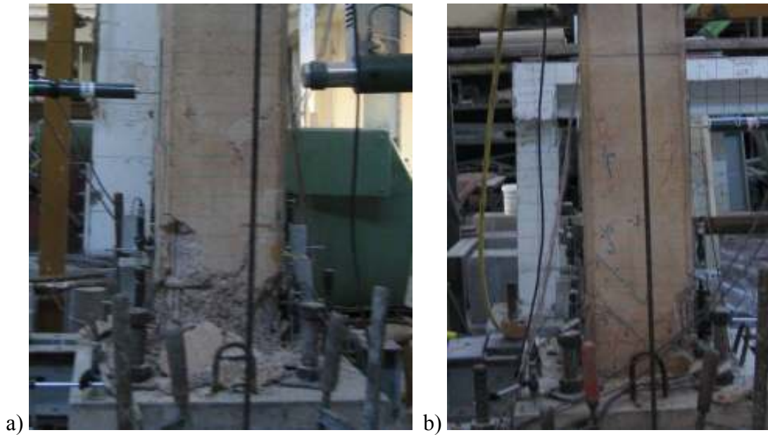
Figure 6.29 : a) North, and b) South view of the LS-X8 specimen after -4.00% drift ratio.
