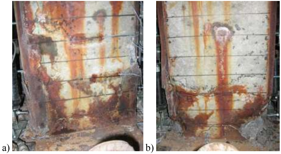
Figure E.293: a) North, and b) South view of NS-X54 after -3.5% drift ratio.
