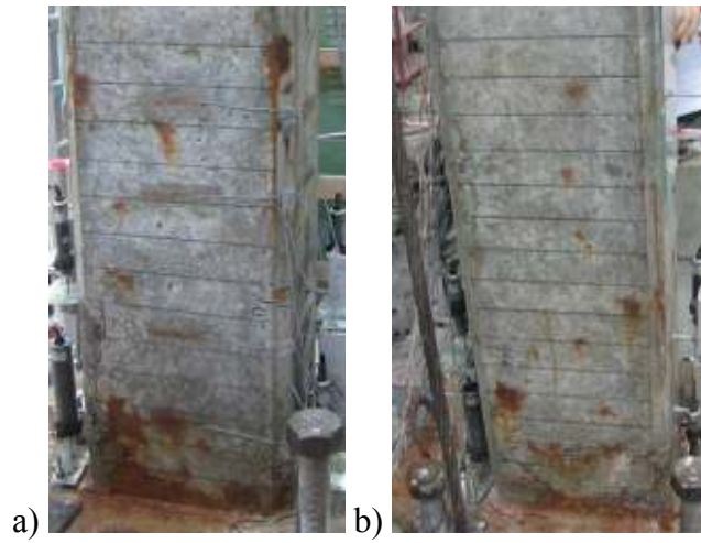
Figure E.257: a) North, and b) South view of NS-X22 after -1% drift ratio.
