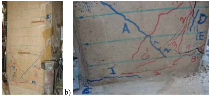
Figure E.55: a) North, and b) South view of LS-X8 after -2.5% drift ratio.
