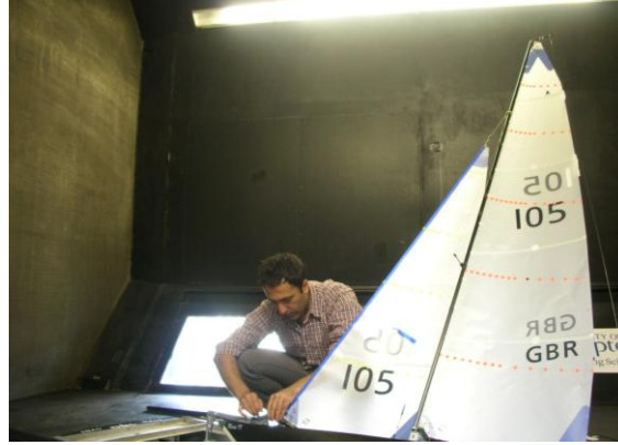
Figure 4.8 : Adjusting twist angle of jib sail in the wind tunnel.
