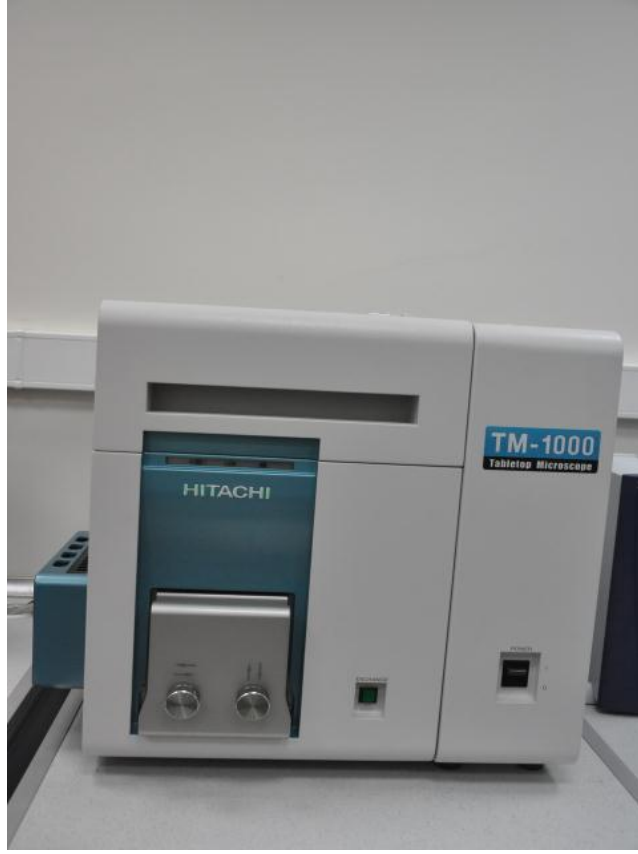
Şekil 3.7 :Hitachi™ TM1000 (Table Microscope)
