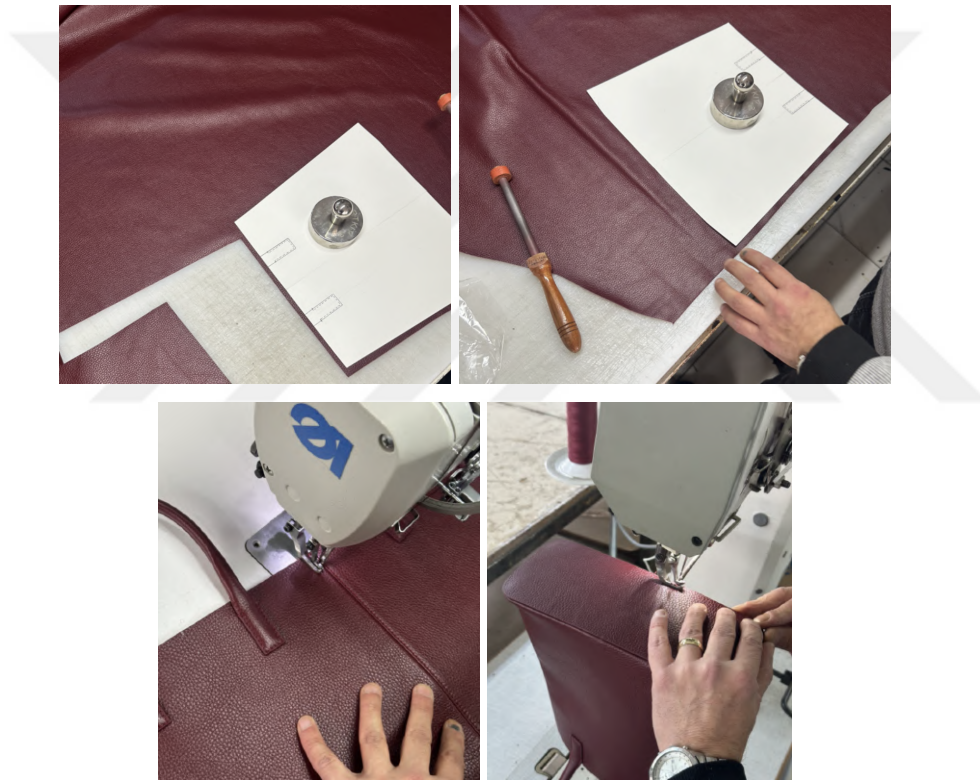
Figure 3.2. Cutting and Sewing Stages of Chrome Tanned Calfskin.
