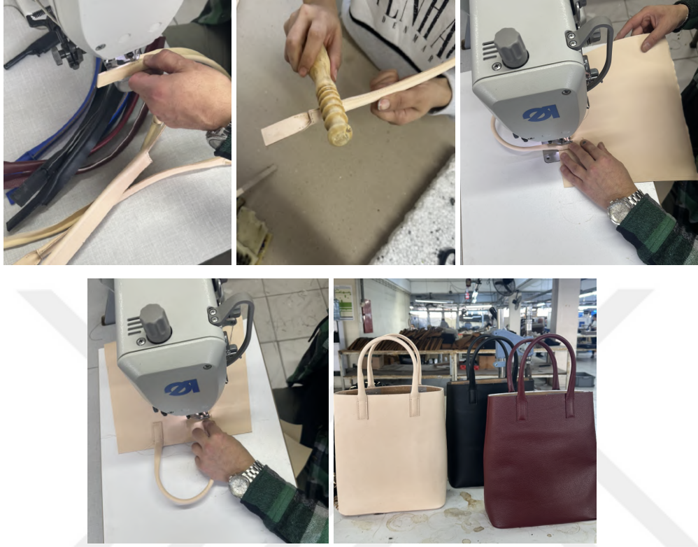
Figure 3.3. Cutting and Sewing Stages of Vegetable Tanned Calfskin.
