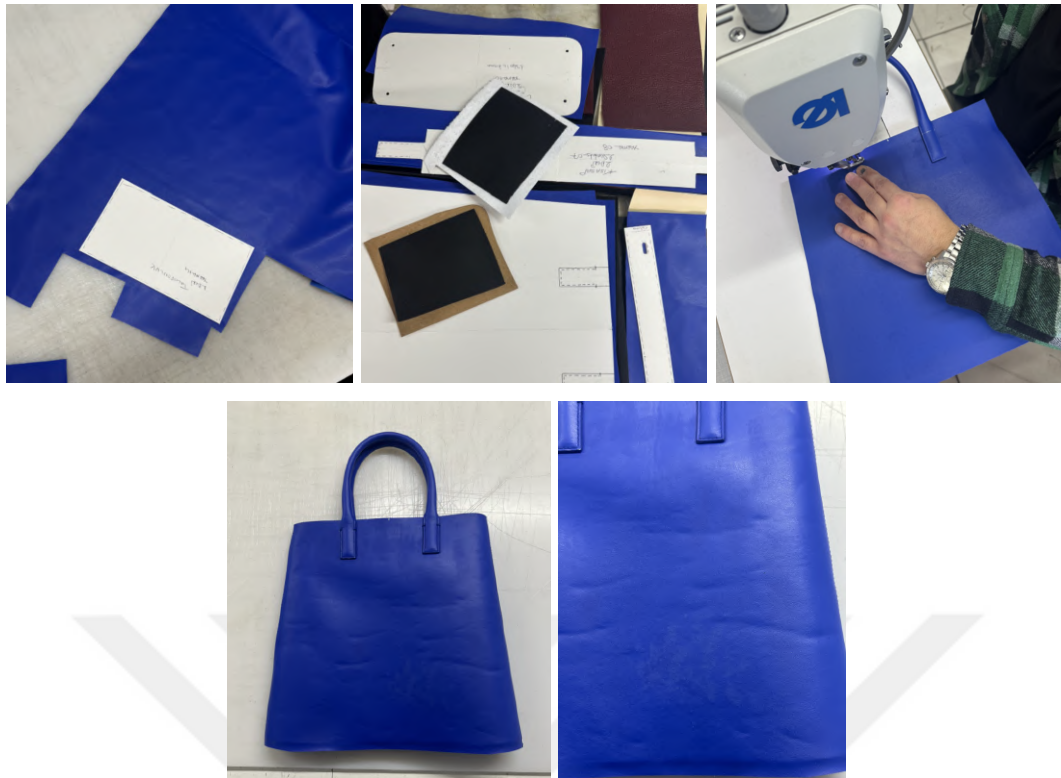
Figure 3.4. Cutting and Sewing Stages of Synthetic Leather.
