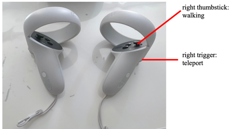
Figure 4.9 : The functions of the buttons used during the experiment on the controllers.
