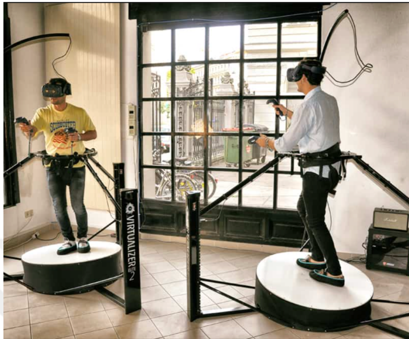
Figure 3.6: iVR setup with an HMD, controllers and the equipment that provides physical movement (URL 2).
