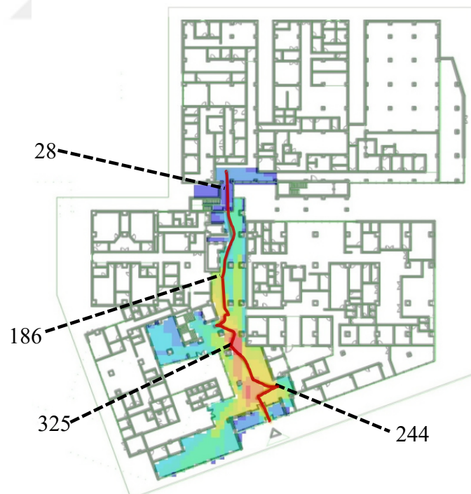
Figure 5.3 : Selected Example: The motion map of Task 1 of P3 and the visibility map of Pars Hospital ground floor overlaid. Examples of the point V values on the route are shown.
