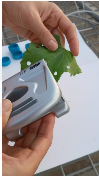
Figure 2.11. Five small discs (approximately equal size) punched from each third leaf to assess RMP.
