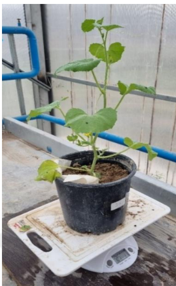
Figure 2.9. A pot weighed before irrigation to estimate water loss.
