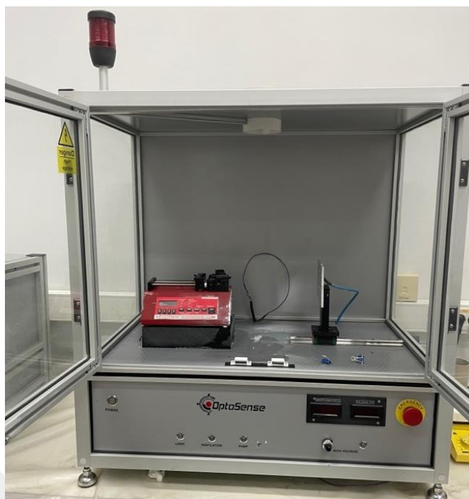
Figure 3.3: Electrospinning device used in electrospinning studies.
