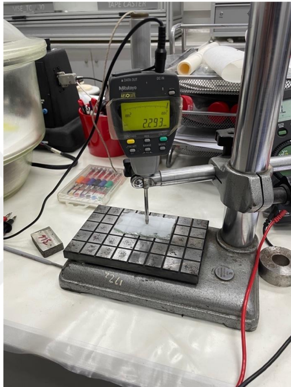
Figure 3.6: The thickness measurement setup
