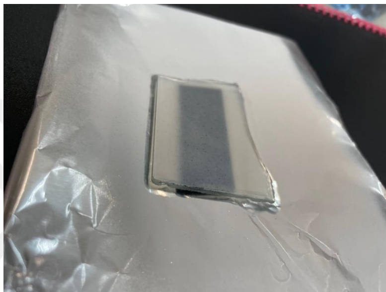
Figure 3.5: Thin film coating of nanofibers obtained from 10 wt.% Ag-PVA on ITO glass.
