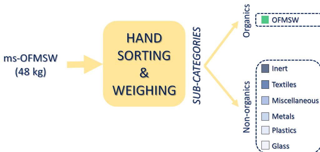
Figure 3.2 : The procedure for determination of waste composition.
