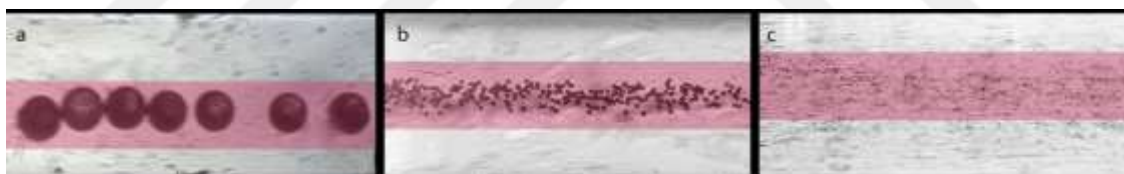
Figure 63. Comparison of PSMs with different sizes; A) 200 \mu\text{m} , B) 20 \mu\text{m} , and C) 5 \mu\text{m} with 100x dilution ratio.
