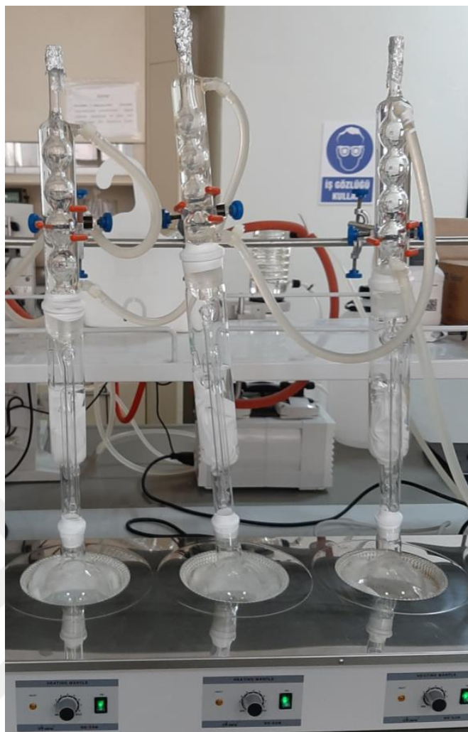
Figure 3.5. Pre-cleaning with Soxhlet system
