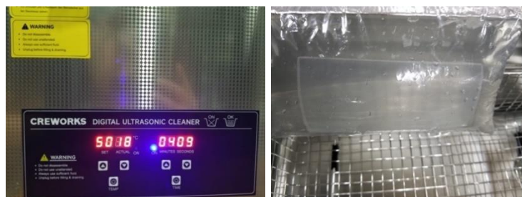
Figure 7.8 : The sample is cleaned in the Crework ultrasonic cleaning device for 25 minutes.
