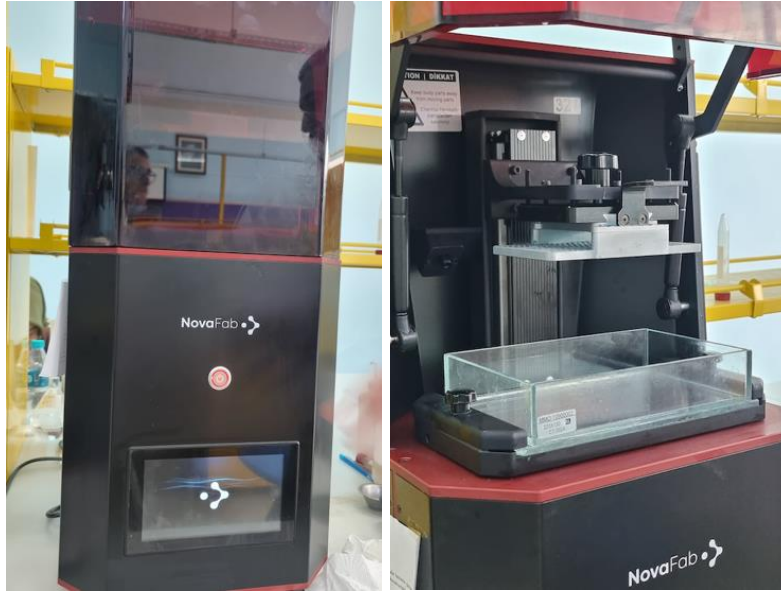
Figure 5.15 : View of the NovaFab DLP device we produce (left), the instrument tank and the build platform (right).
