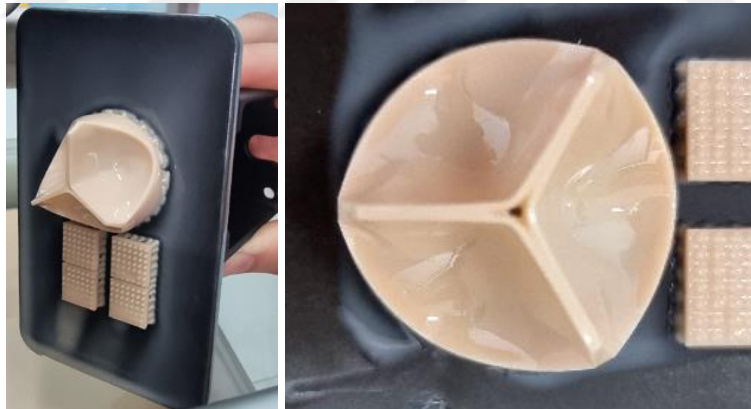
Figure 5.16 : View of the model we produced with DentaModel on the platform of the DLP device (left) and top view of the model (right).
