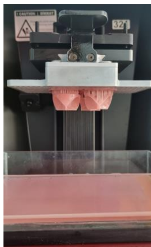
Figure 5.18 : Post-printing view of the valve model we printed on the platform.
