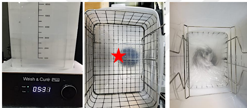
Figure 7.7 : The test specimen is cleaned in water in the Anycubic wash&cure device for 5 minutes. The test sample is where the star symbol is.
