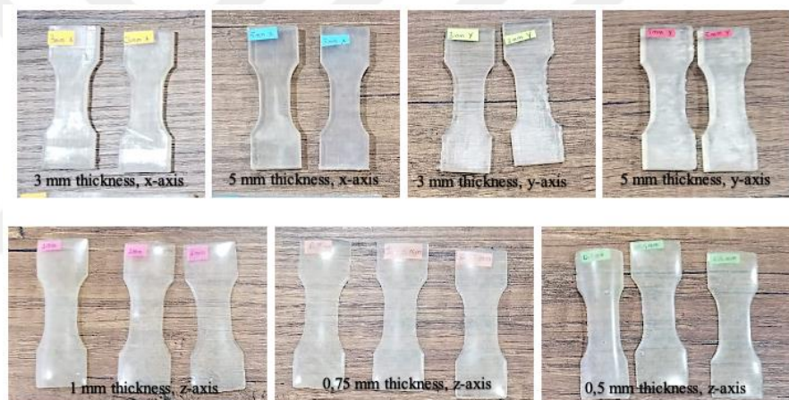
Figure 7.10 : Specimens for the uniaxial test. The thickness and compression axes of the specimen are given in the images.
