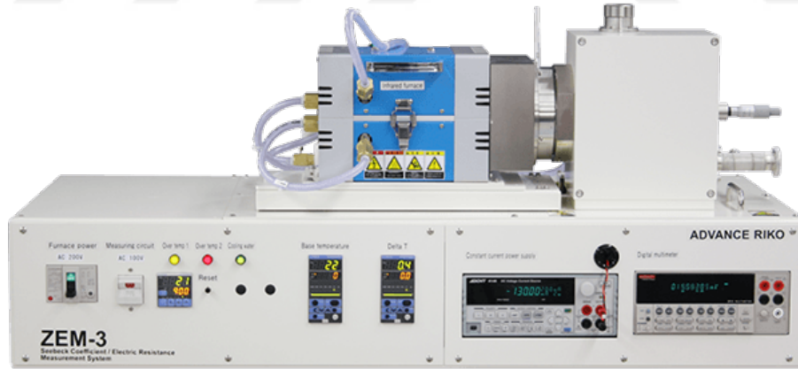
Figure 4. 8 Electrical resistivity and Seebeck coefficient measurement system.
