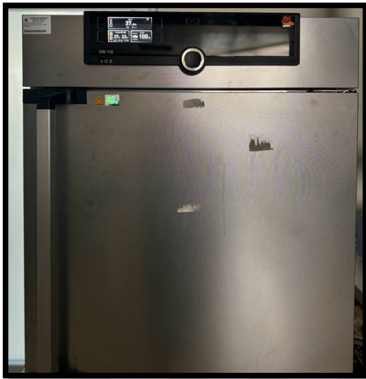
Figure 12. The incubator used to keep the specimens at 37^\circ\text{C} .
