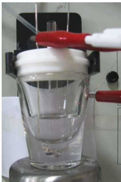
Figure 2.2: Cell Which Is Used At The Electropolymerization
