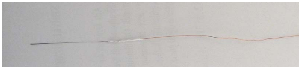
Figure 2.1 : Carbon Fiber Micro Electrode
